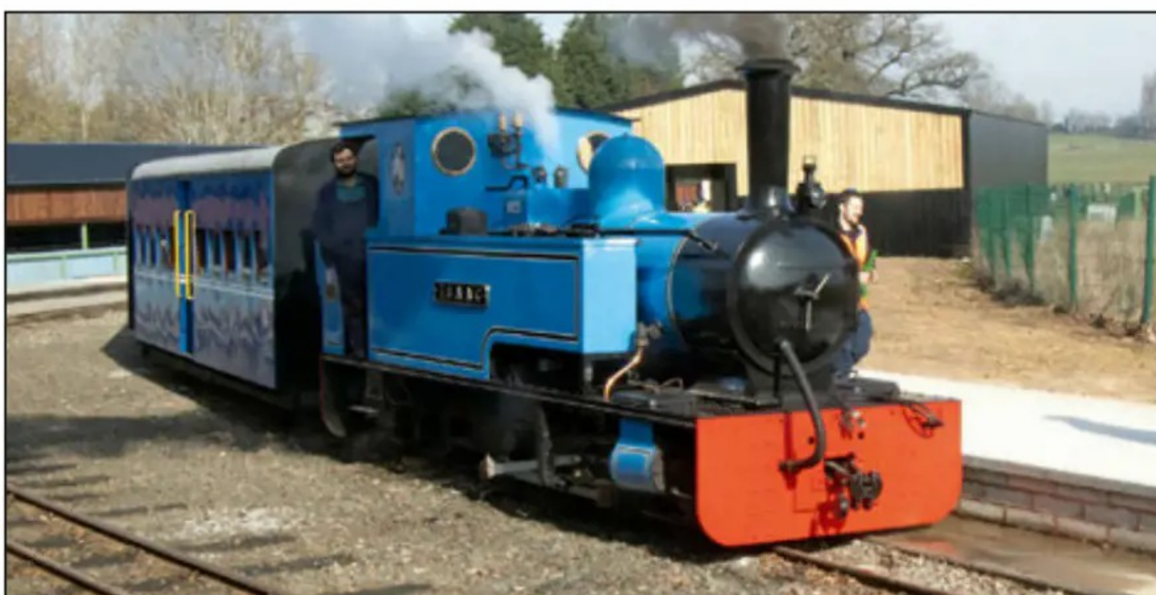
■ 'Handy Man', the 3ft gauge Hudswell Clarke 0-4-OST (573) built in 1900 for the Burton Ironstone Company, has taken up residence at the Statfold Narrow Gauge Trust following the loco's cosmetic restoration at Workshop X in Killamarsh, Derbyshire.
