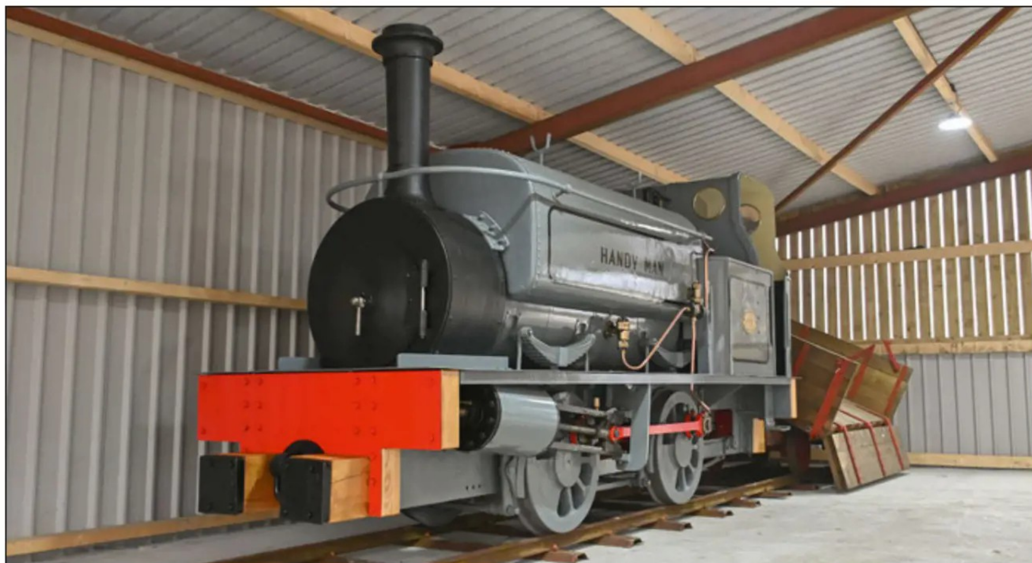
■ 'Handy Man', the 3ft gauge Hudswell Clarke 0-4-OST (573) built in 1900 for the Burton Ironstone Company, has taken up residence at the Statfold Narrow Gauge Trust following the loco's cosmetic restoration at Workshop X in Killamarsh, Derbyshire.
