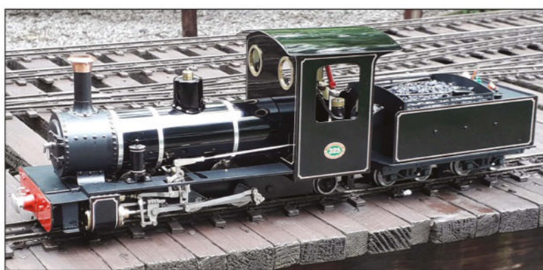
Right: Superb 16mm scale live-steam model of 2-6-2 'Black Beauty' in original condition before it was named. It was built by a skilled enthusiast in Yorkshire. Photo: James Waite collection
