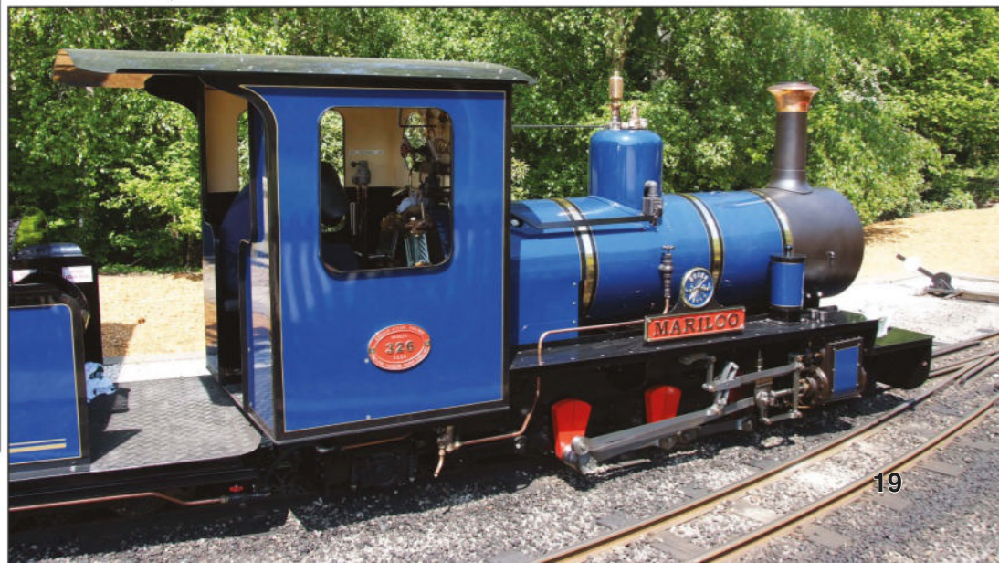
Below: 12¼in 2-6-2 'Mariloo' stands at Exbury Central station on 8th May 2008, five days after delivery from Exmoor and four days after it was named by the late Queen. Note the smart style of numberplate, also applied to 'Black Beauty'.
