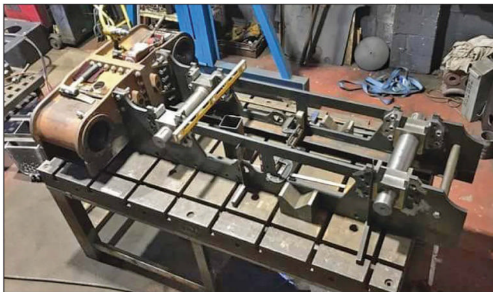
Below: Significant progress – the very latest photo from NBRE shows the cylinders mounted on the chassis, which in this picture is upside down on the workbench. Photo: NBRE
