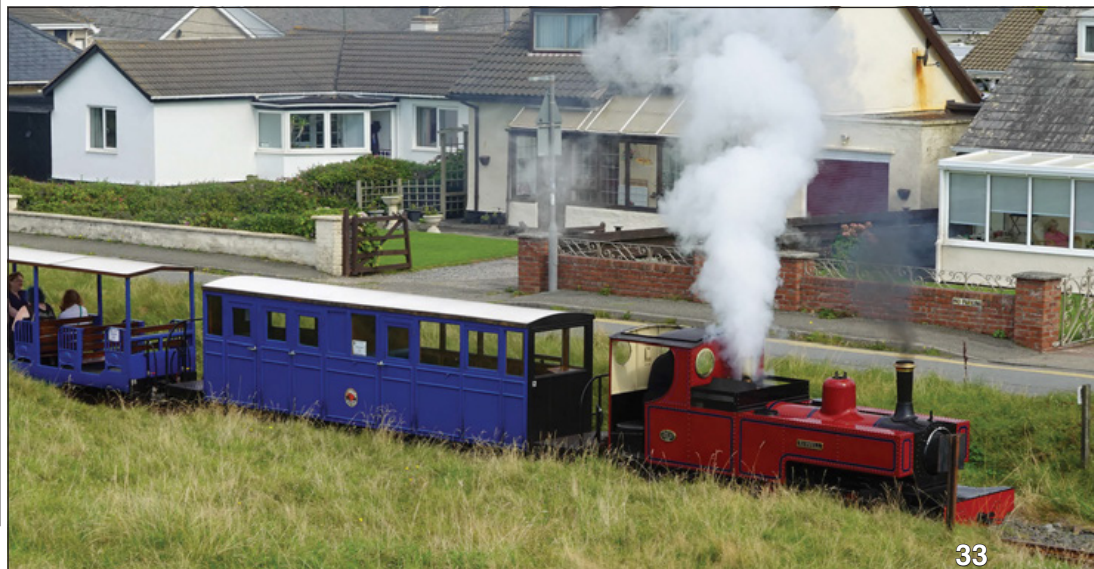
Below: More first-generation briquettes in September 2021 on the Fairbourne Railway. 'Russell' was running well enough, but the dark smoke is a clear indicator of incomplete combustion – even though the safety valves are lifting.
