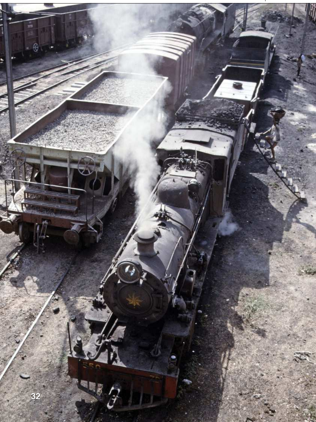
2-8-2 TYPE 38½-TON TENDER LOCOMOTIVE IN SERVICE ON THE 2' 6" GAUGE BARSII LIGHT RAILWAY, INDIA (Further details near)
