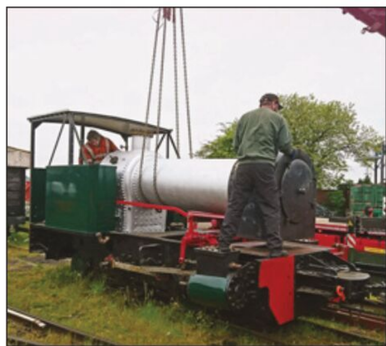
■ Restoration of the Sittingbourne & Kemsley Light Railway's Kerr Stuart 0-4-2ST 'Premier' (886/1905) passed a milestone on 13th May when the boiler was returned from NNR Engineering at the North Norfolk Railway and reunited with the boiler. The S&KLR reopened on 2nd May and is running on Sundays throughout June. Photo: Liz Fuller/S&KLR
