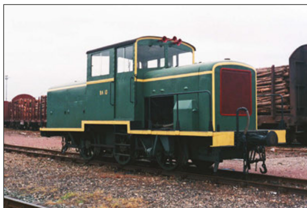
Locotracteur BA13 on the sidings at Salbris on 22 June 1994. Its twin BA14 was also seen in the loco depot. The two were used on freight and latterly for works trains. They were built on the chassis of two 1901 Blanc Misseron steam locomotives in 1953.
