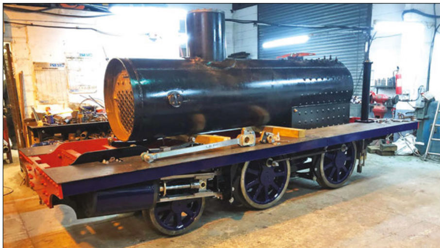
■ The project to recreate the former Southwold Railway Sharp Stewart 2-4-0T ‘Blyth’, scrapped in 1941, took a major step forward at the end of November when the boiler was trial-fitted onto the chassis. David Humphreys of North Bay Railway Engineering Services, which is building the loco at its Darlington workshops, told NGW that the smokebox and chimney are ready to be installed and Blyth could now effectively run on compressed air. The Southwold Railway Trust is currently raising the around £80,000 required to finish the engine – donations can be made through its website at www.southwoldrailway.co.uk/trust-projects/2-4-0t-no-3-blyth/ Photo: NBRE
