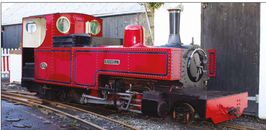
■ The Fairbourne Railway’s Milner 12.25-inch gauge locomotive ‘Russell’, built in 1979, has emerged from the line’s paint shop in a new version of its red livery skillfully lined out in two shades of blue. Unlike its 2ft gauge 2-6-2T inspiration at the Welsh Highland Railway the Fairbourne Russell is a 2-6-4T, due to the loco originally being built as a representation of the Leek & Manifold Railway locos. Various issues, including a tiny cab, led to a rebuild into its present form in the Fairbourne workshops in 1985. Photo: FR
