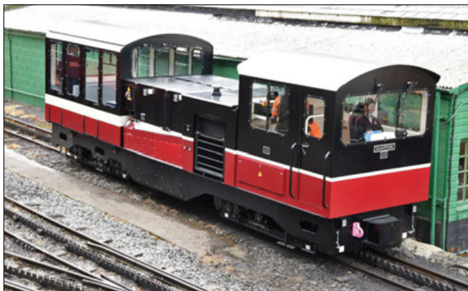
■ The Snowdon Mountain Railway has revealed the final appearance of its two new hybrid-electric locomotives, following the delivery of the 12-seat passenger pods that are attached to the front of each. The locos, built by Clayton Equipment Ltd, have also been named – no 14 on the line's roster takes the name 'Glaslyn' after the lake around 600 metres (2000ft) above sea level which can be seen from the summit on the eastern sides of Snowdon, and no 15 is to be called 'Moel Eilio', which is a 2382ft high mountain around three miles north-west of Snowdon. The SMR reopened on 10th July, running only to its highest intermediate station of Clogwyn for the 2020 season. Photos: Peter Johnson
