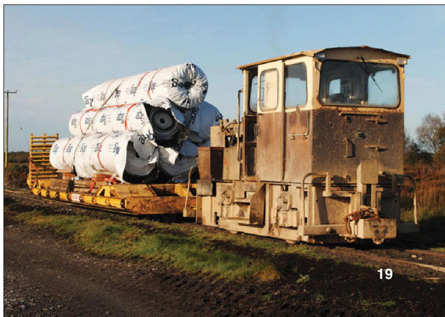
Right: There can be many surprises on the BnM. What looks like a load of giant carpets is degradable track underlay used on virgin bogs where the ground is soft. LM 400 is at the Derelahan triangle on the Blackwater system. Photo: Paul Carpenter, October 2017
