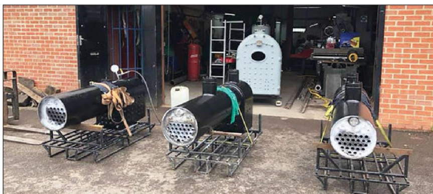
■ An impressive picture from North Bay Railway Engineering Services on 9th July, with some four newly-built boilers lined up in the workshops ready for ultimately successful boiler tests. The large one to the rear is destined for the project to build a modern recreation of the Ffestiniog Railway's lost England 0-4-0 'Mountaineer' while the others are for a 6-inch Burrell road loco and two miniature locos for a private client.
