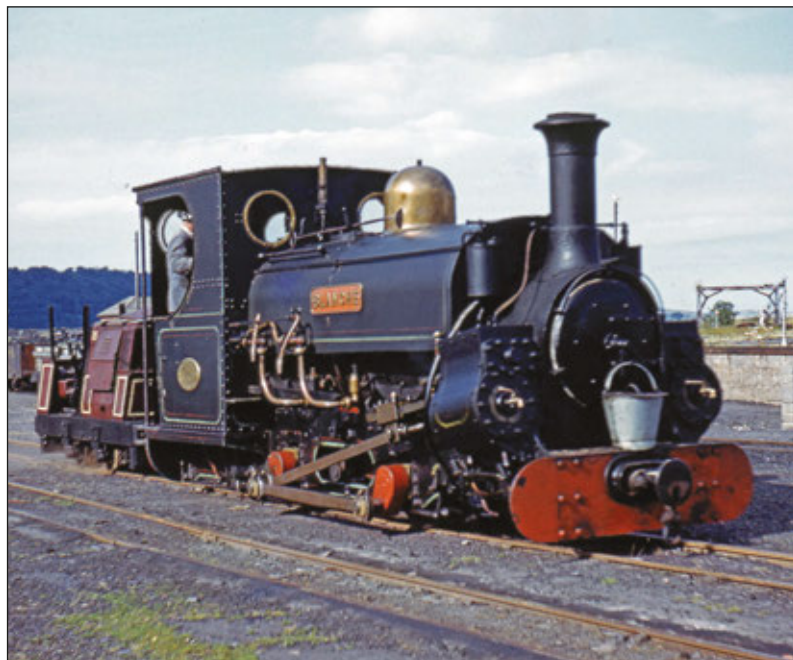
Left: 'Blanche' at Port Penrhyn about to bump-start diesel no 23. The sand bucket hung on the front was a feature of Penrhyn mainline engines. Photo: R L Mitchell
