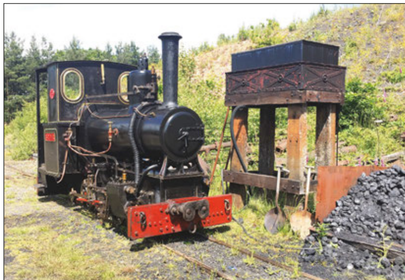
Left: Barclay 0-4-0WT 'Glyder', restored in 2019, retains much original paintwork as a result of great care to preserve the working patina acquired at Penrhyn Quarry. It rests alongside the suitably industrial water tower and coal platform. Photo: Paul Jarman
