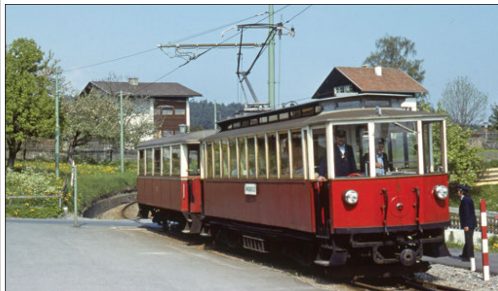
Above: Stubaital no 2 (Graz 1904) entering Mutters with a Fulpmes to Innsbruck train. It is towing no 15, a four-wheeled trailer rebodied in 1966 and withdrawn in 1982. It went to the museum tramway at St Florian, near Linz.
