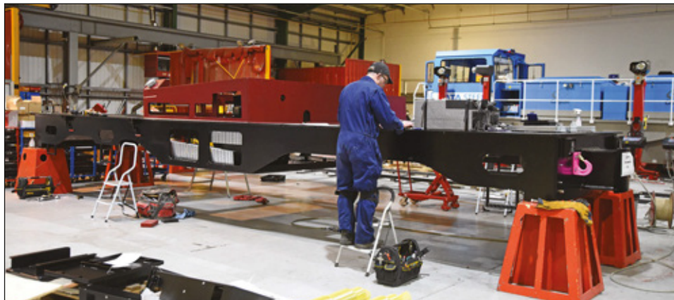
■ First photos have emerged of the two new 800mm hybrid electric locomotives being built by Clayton Equipment Ltd for the Snowdon Mountain Railway. No general arrangement drawings have yet been published but it is clear from the main picture that they will be very long locos. NGW understands that this is because each one will include a 12-seat passenger pod on its front end. Photos: Peter Johnson
