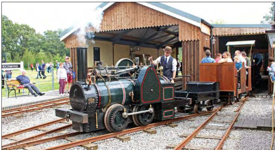
■ This year's annual open day on the private Richmond Light Railway in Kent on 17th August featured Beamish Museum's new-build Thomas Green loco 'Samson'. The loco is seen here departing from the line's impressive station with a shuttle train, topping and tailing with vertical-boilered 0-4-0 'Leary' recently acquired by the Richmond line. We'll have more on this delightful 2ft gauge line next month.
