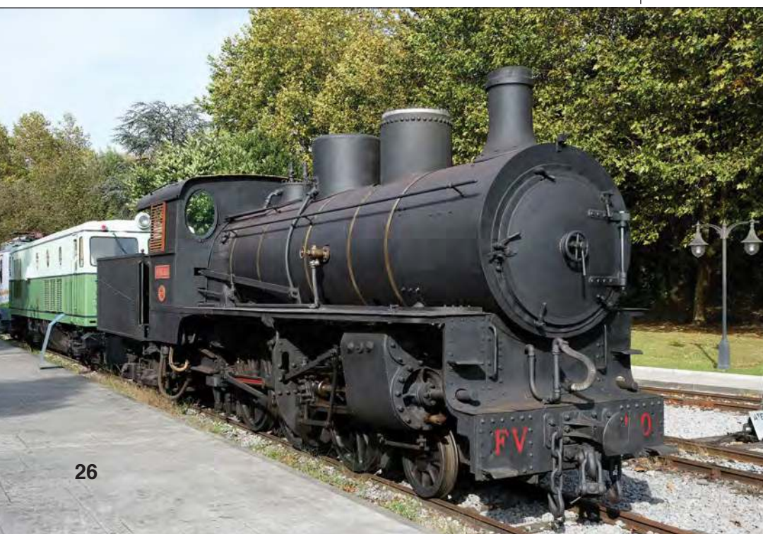
Below: Awaiting overhaul is FV 2-6+4 Engerth no 56 'Urko'. It has been restored as class-mate no 50 'Euskadi' – the local name for the Basque country.
