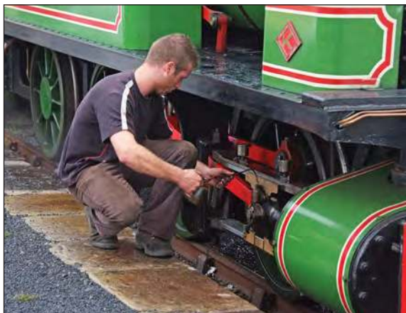
Above: Oiling the motion of Slieve Callan before departure. Photo: James Waite
