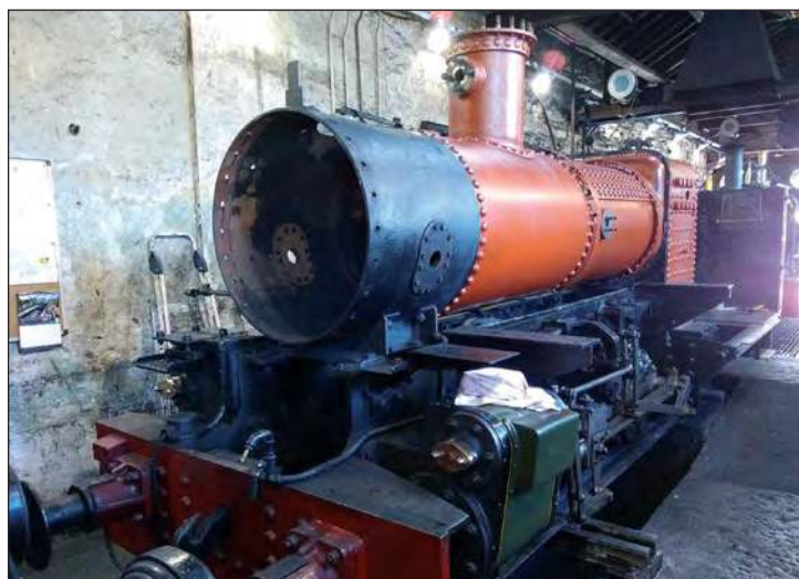
■ Winter work at the Talyllyn Railway includes a major overhaul of 0-4-2ST 'Tom Rolt' built by the railway and first entering service in 1991. This was the scene at Pendre works on 17th October with the loco already stripped down. Photo: Chris Smith/TR
