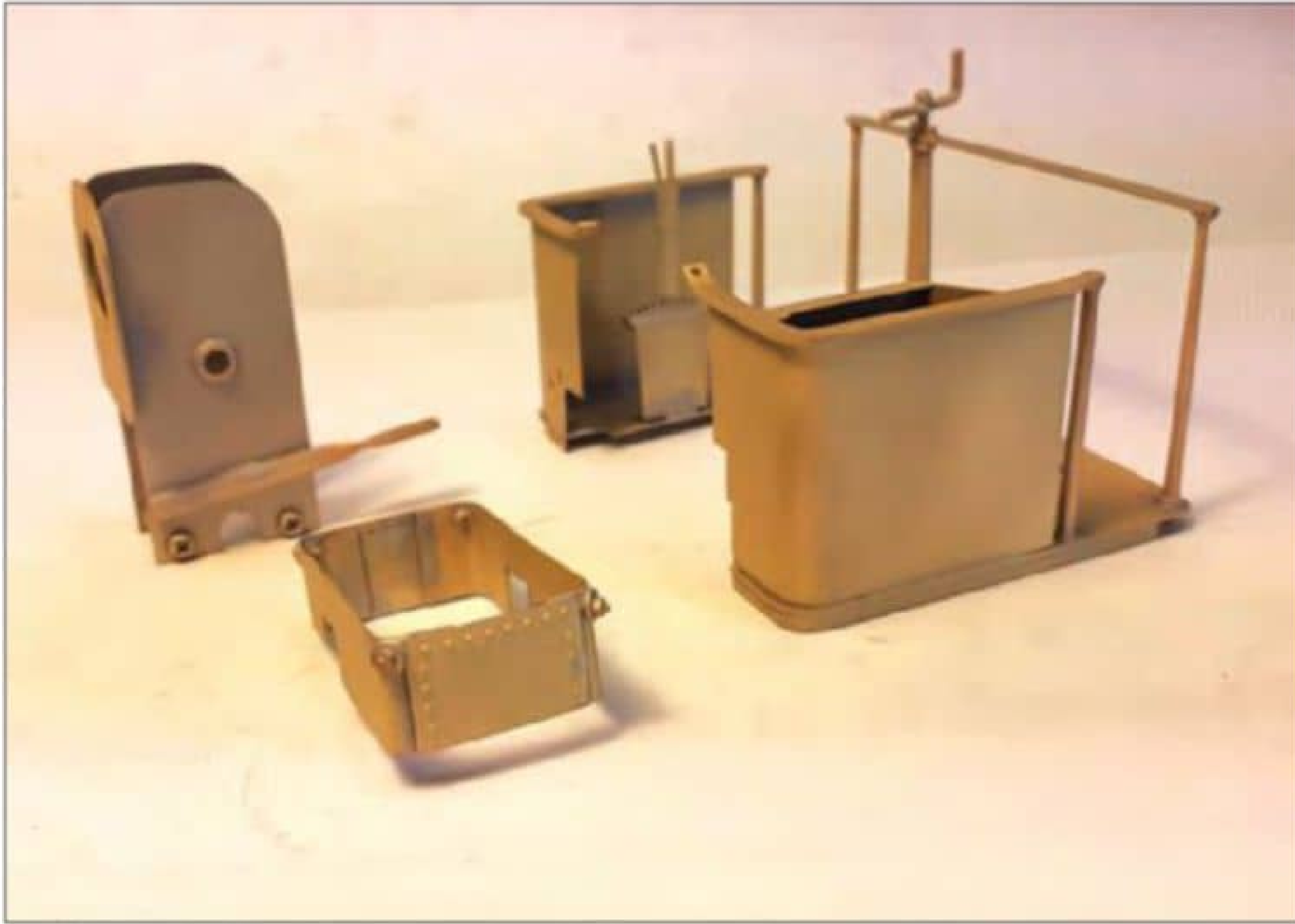
9. The Cab floor with bunkers, the ashpan and the gearbox casing.
