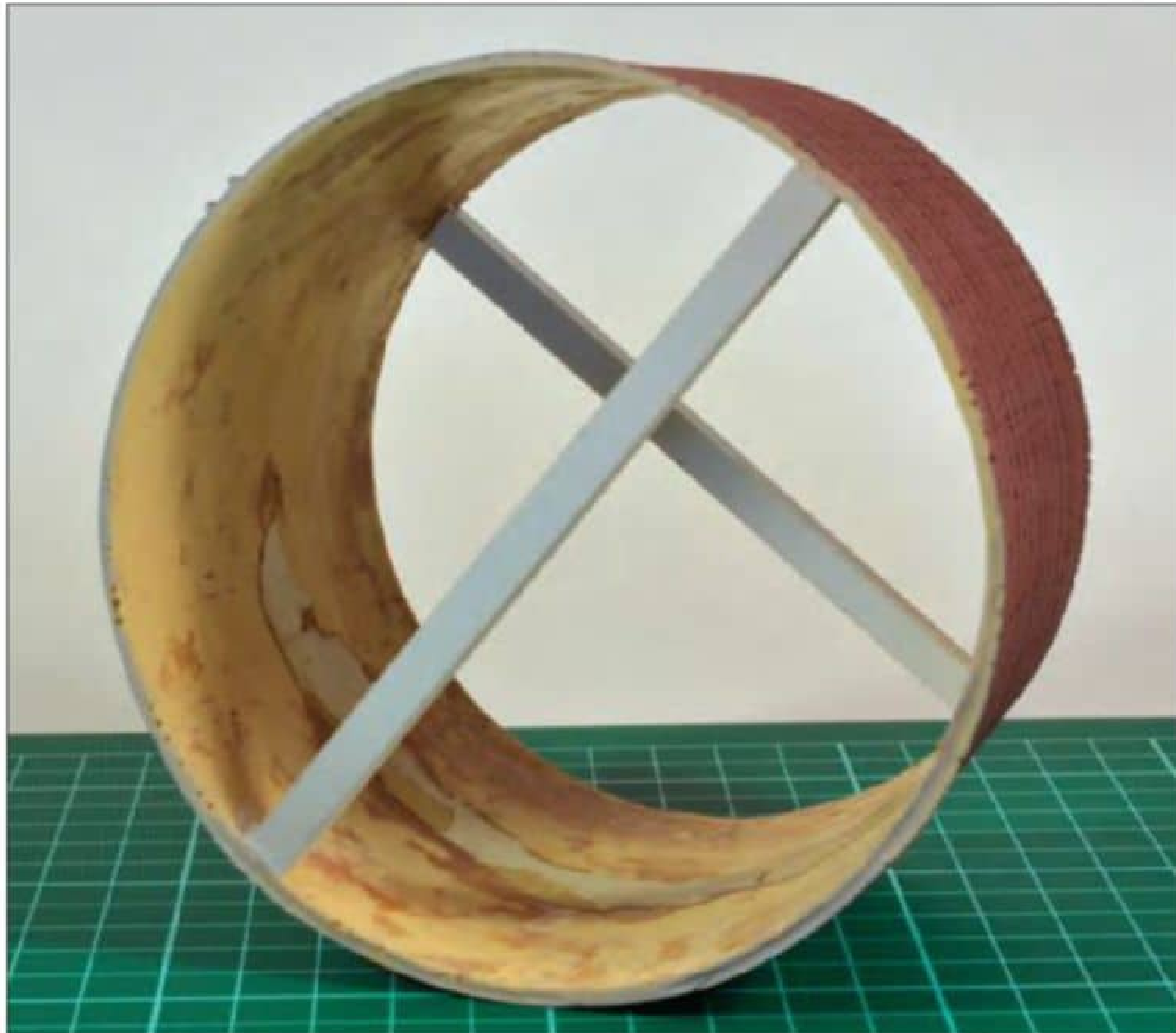
Tank casting with some supports added from square styrene to maintain the tank shape.
