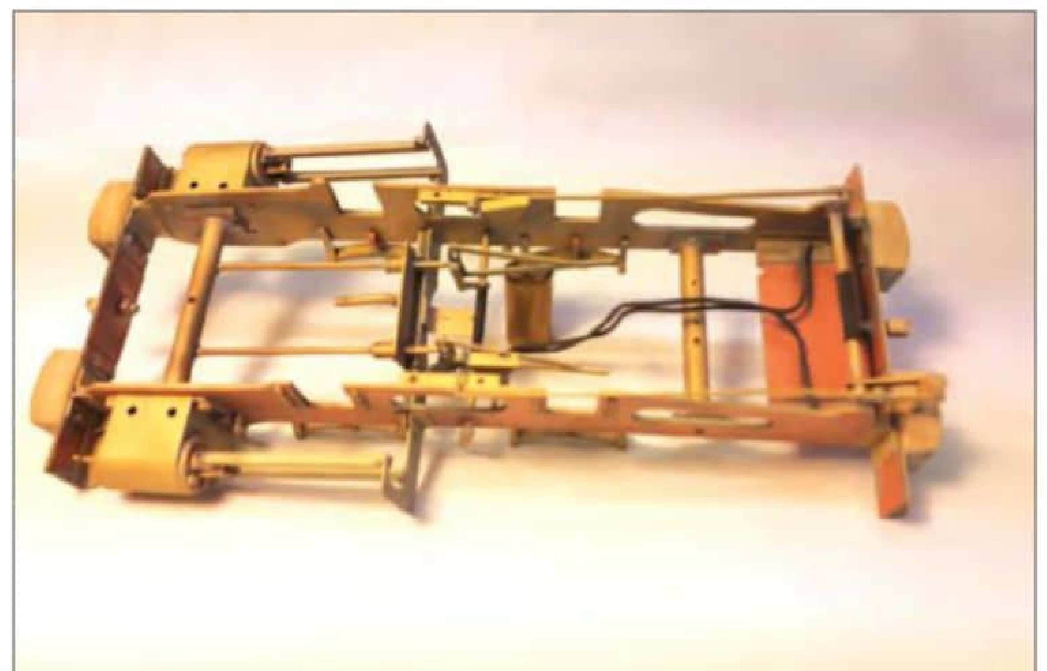
2. The chassis underneath showing dummy valve gear
