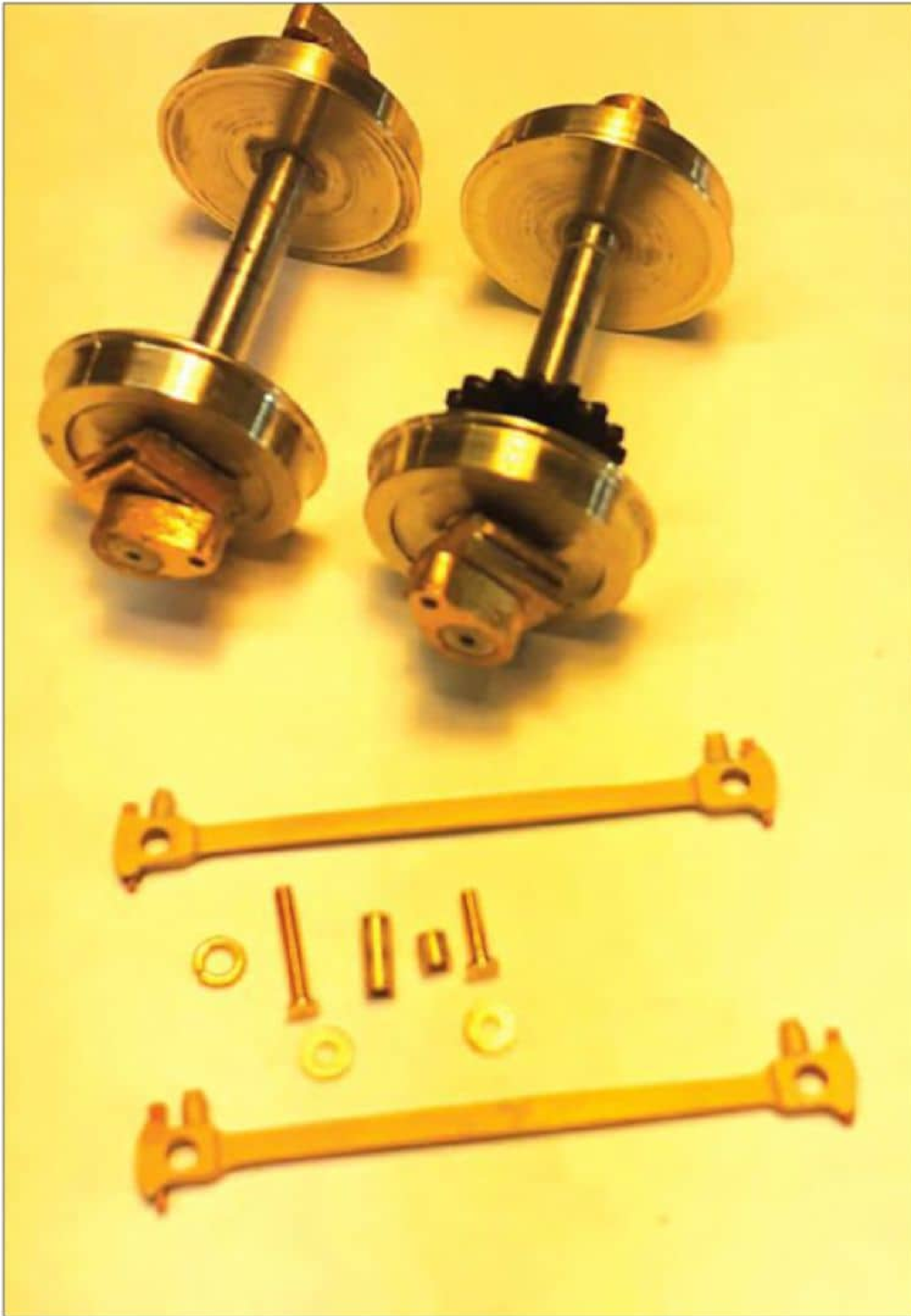
Left 3. Assembled wheelsets, rods and crank-pins.
