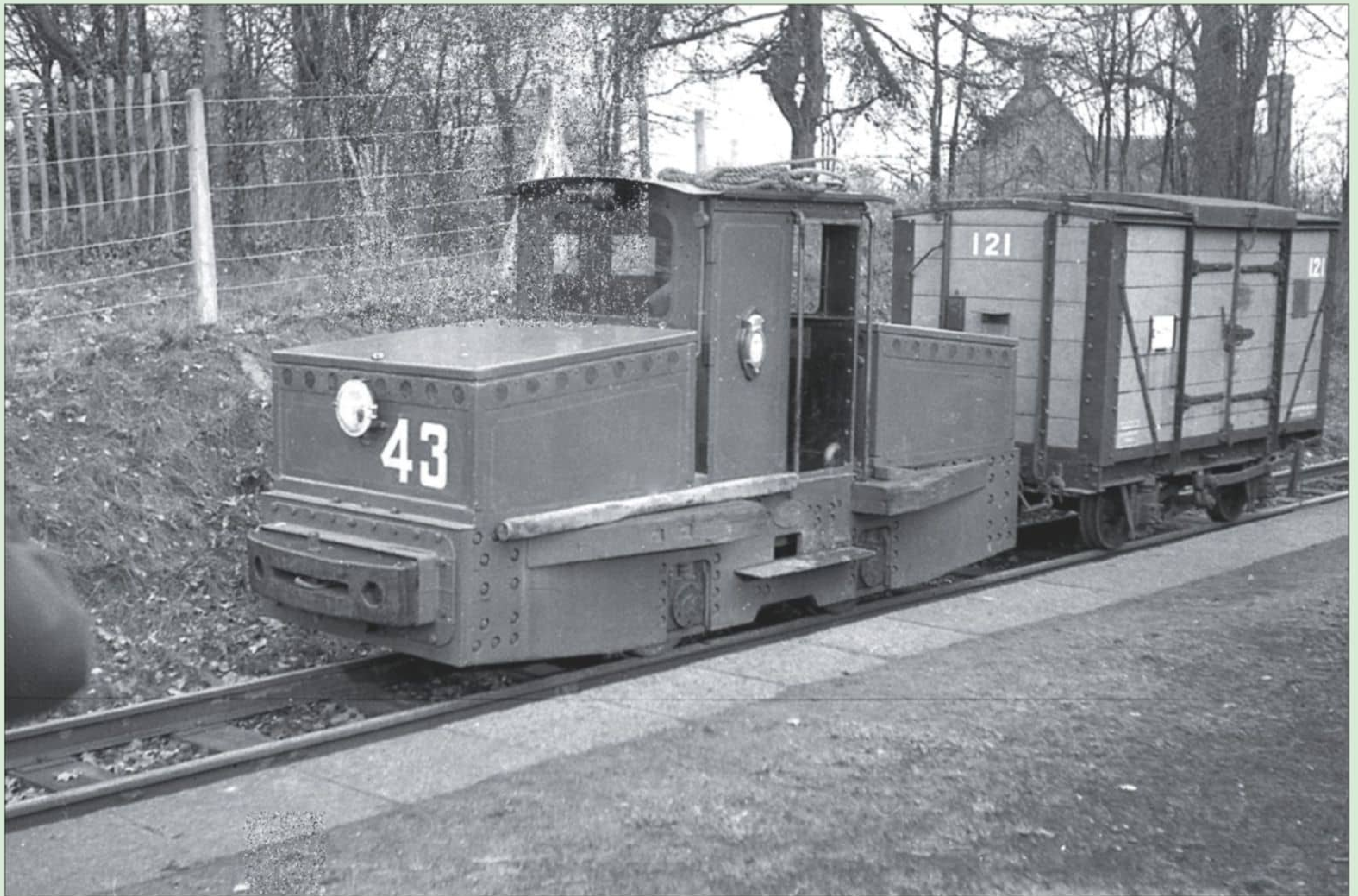
At our request, one of the dockyard battery locomotives, 43, Greenwood & Batley 1581 of 1938, followed 107 out of the dockyard so we could photograph it.
