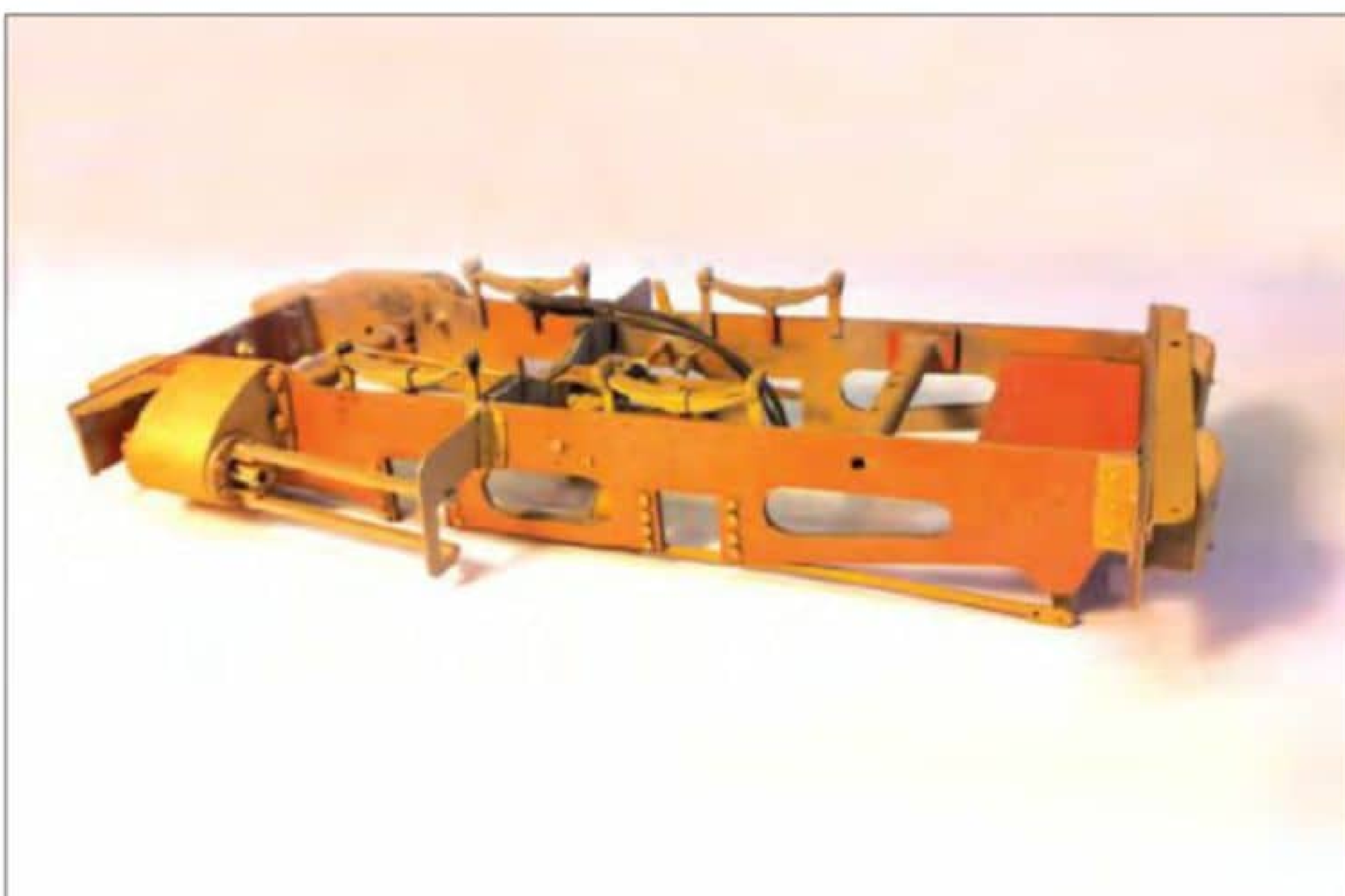
1. The chassis, sandblasted and ready to paint.
