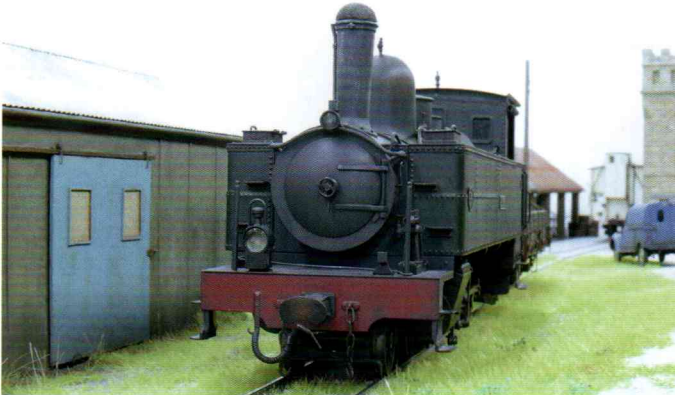
Above: Twelve of these 4-6-0s were built between 1904 and 1909 – this one, E332, being the last built by Compagnie Fives-Lille. The model was built over thirty years ago from nickel silver and, although it is built from scratch, I did draw, and have photo etched, the valve gear and motion parts. The re-railing jack, carried by all engines on the Réseau Breton, is a 7mm scale S&D Models casting, but it doesn't look out of place on these 1:50 models.
