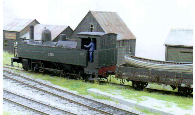
Above: Twelve of these 4-6-0s were built between 1904 and 1909 – this one, E332, being the last built by Compagnie Fives-Lille. The model was built over thirty years ago from nickel silver and, although it is built from scratch, I did draw, and have photo etched, the valve gear and motion parts. The re-railing jack, carried by all engines on the Réseau Breton, is a 7mm scale S&D Models casting, but it doesn't look out of place on these 1:50 models.
