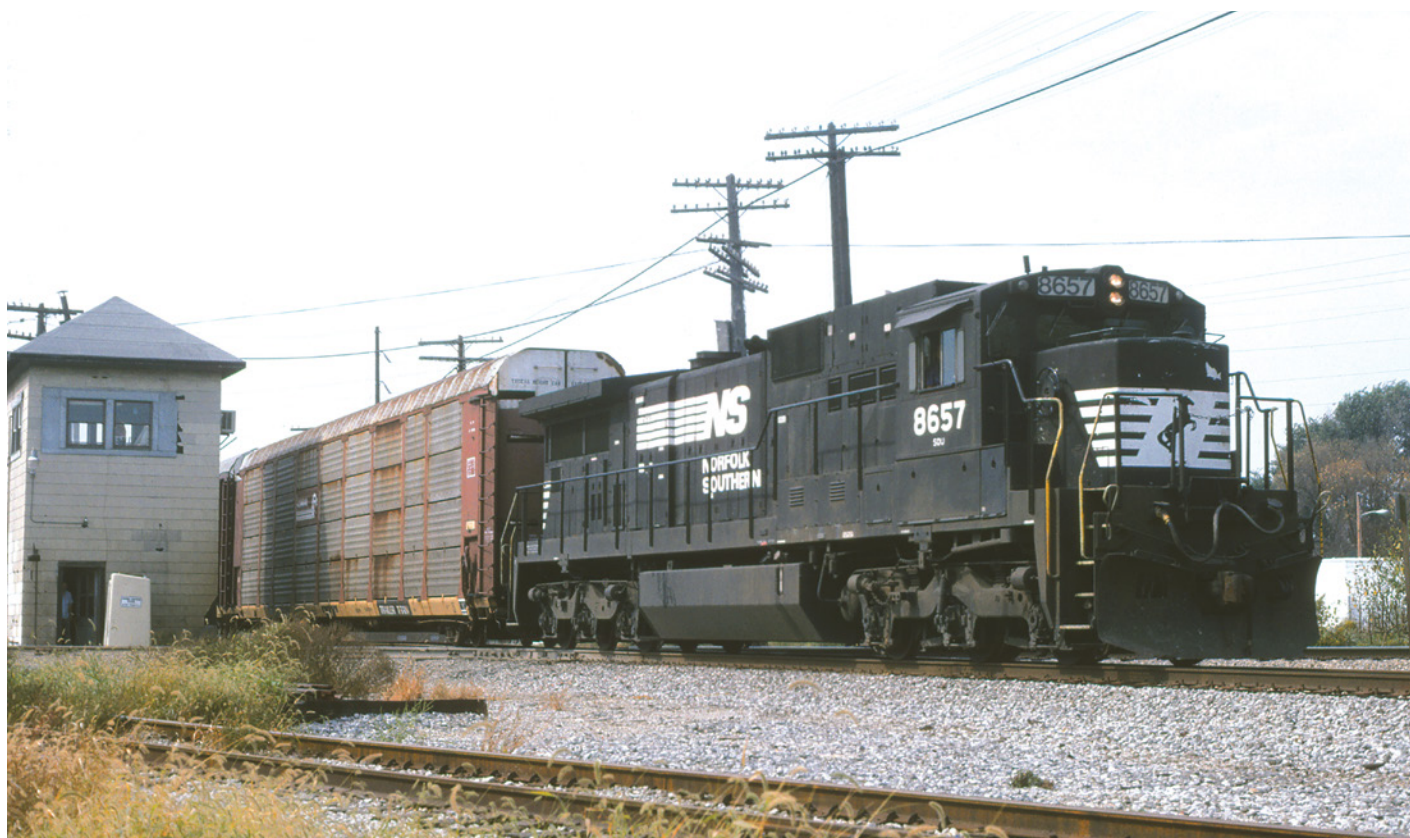
Above: As stated in the introduction, this is the exact scenario I was referring to as Norfolk Southern 8657 leads train 416 past Iles Tower and over the Southern Pacific diamond on the south side of Springfield, Ill., on October 8, 1993. NS 8657, built in October 1986, represents a Phase III C39-8, constructed in the same order as the review NS model. General Electric C39-8 Phase III details include a wheel handbrake on the side of the short nose, lack of a headlight knockout on the front of the nose, classification lights, exhaust stack extension, GSC trucks, 4,400-gallon fuel tank, and a large plow. ScaleTrains.com has meticulously included these details on its new Rivet Counter HO-scale offering. It's as if they knew I was going to write a detailed HO-scale model review exactly 25 years after I photographed this unit in Springfield. —Ryan Crawford photo
