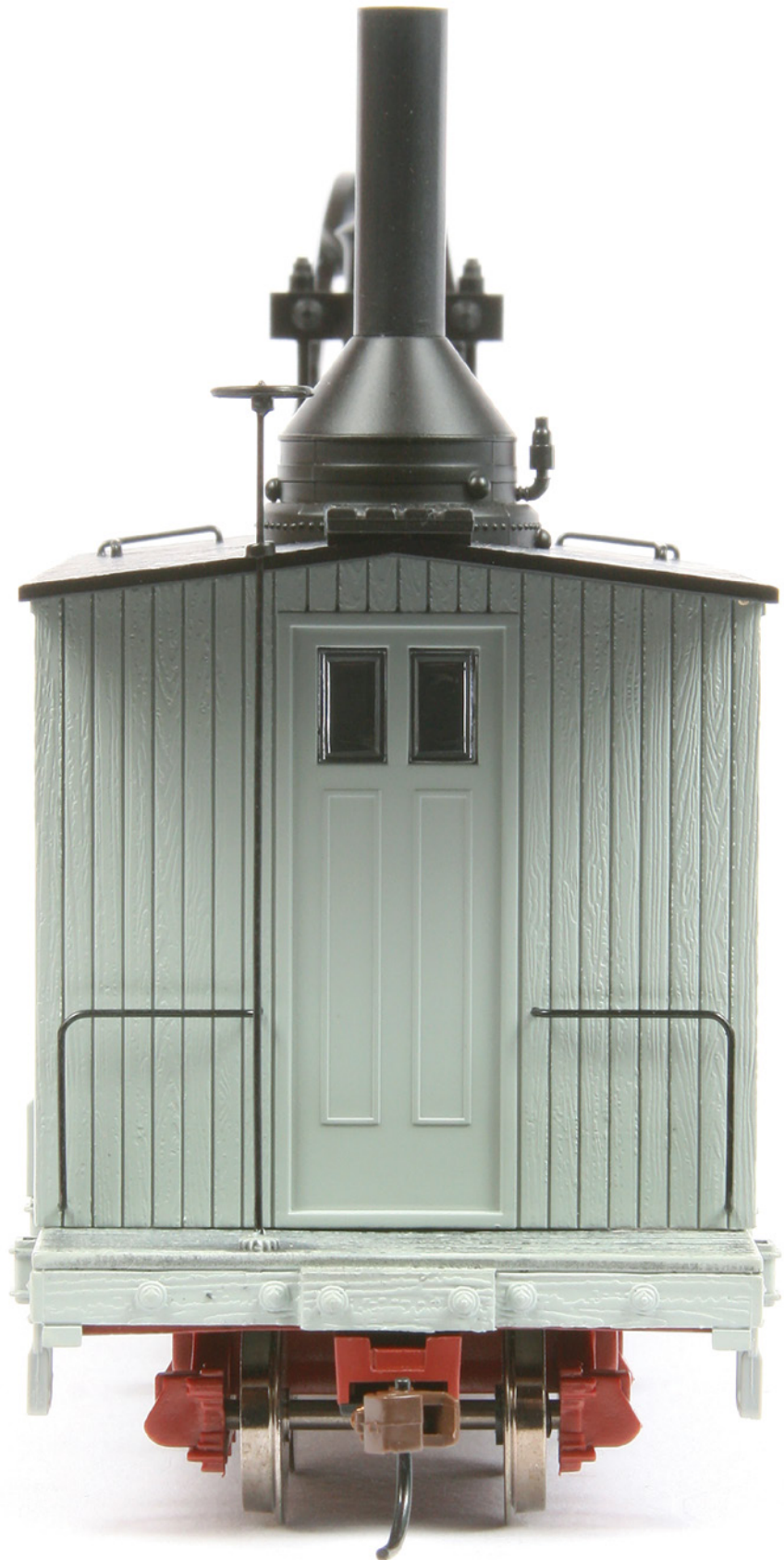
Above: The non-business end of the car is functional, yet plain. There should be a ladder here as well, otherwise the brake wheel is less useful. I plan to shorten the brake staff to a height that a crew member could stand and operate from the deck of the car. The derrick car is built on the manufacturer's existing On30 flatcar tooling. The model's flatcar base and crane equipment house come molded in a gray color with black roof. The underframe and trucks come molded in a rust colored plastic.
