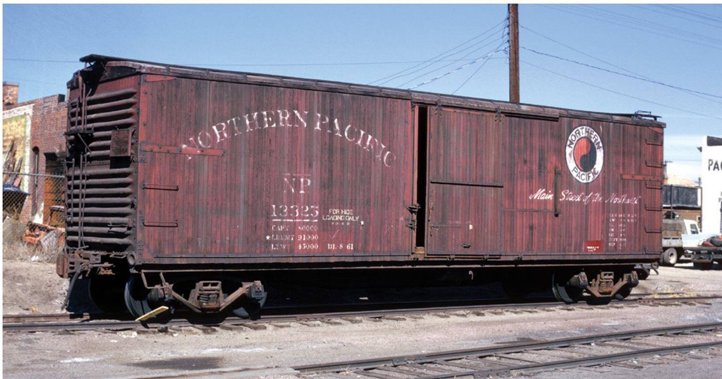
Above: October 10, 1966, finds NP 13325 wearing the final 1951-1956 paint scheme in hide service at Butte, MT. It is still reporting the original road number given at the Pullman Car & Manufacturing Company in 1925. This survivor was one of the last 500 cars in Northern Pacific's 10000 series double-sheathed boxcar order. —Matt Herson photo
