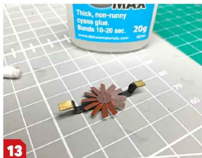
The brass fan was sprayed with red oxide primer then weathered with a dark enamel wash. I had to rig up a mounting bracket from thick brass strip, painted black, which was shaped to allow the fan to sit below the grille.
