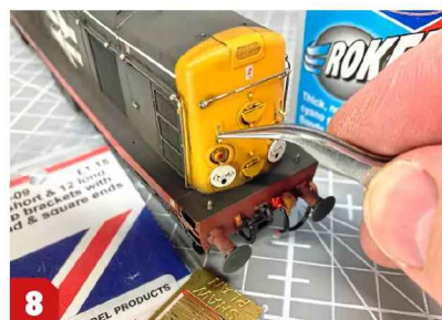
With the initial weathering stage complete, it was safe to install the headcodes disc and bufferbeam detail. I lost the nose-end lamp brackets, so I folded up replacements from Shawplan etched brass strips, slotted into the mounting holes.
