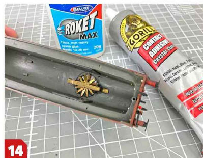
My makeshift bracket was fixed into position with slow-setting cyano glue, so I could check the alignment before it set. To provide a more resilient bond, I then spread some contact adhesive around the joints (a Dave Lowery tip!).
