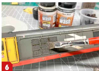
Next day, I decided the side grilles and louvre panels needed extra contrast, so I applied a much darker blend of enamel washes, targeting it more precisely, and only wiping away pigment that had strayed outside the grilles.
