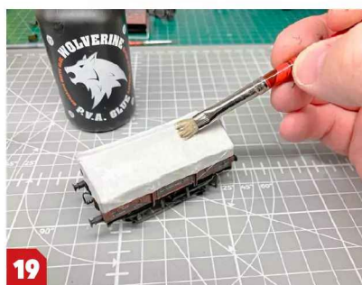
19 Excess glue was wiped away from the wagon body with a swab. I then applied a coat of the same Wolverine glue, diluted slightly with water, brushed lightly over the entire hood.
