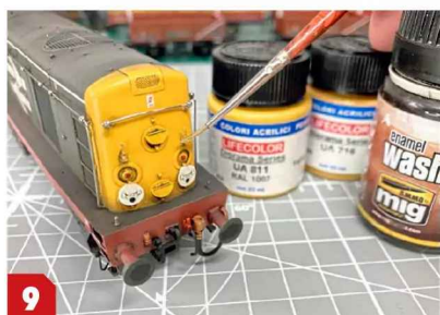
When the glue had set, the brass lamp brackets were touched in with paint (I mixed some LifeColor shades to a close match), then weathering wash was added to help them blend into their surroundings.
