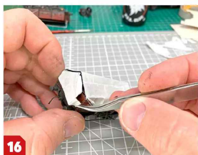
16 The tabs of the end section were folded over and carefully tucked under the main sheet section. I ensured the lower edge of the hood matched up with the sides.
