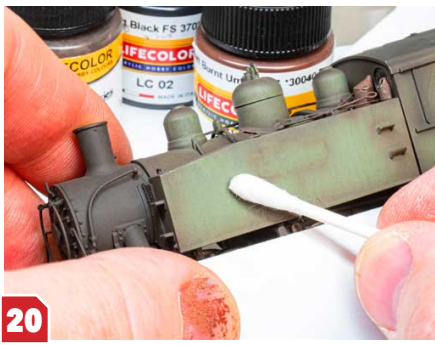
The same blend was applied to the body, one section at a time, wiping it away with vertical strokes to ensure remaining streaks mimicked the action of gravity. Dipping a swab in thinners helped shift stubborn deposits.
