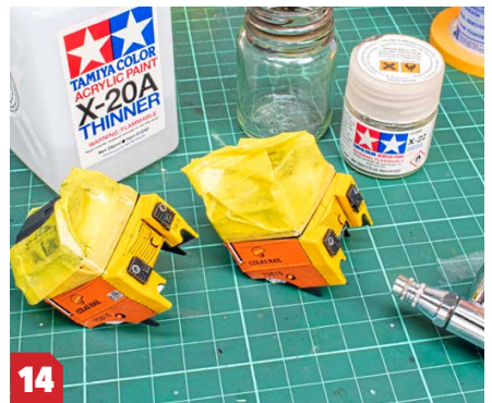
14 To render the decal film invisible, I sprayed a light coat of clear gloss acrylic (Tamiya) via an airbrush. When this was dry, I sprayed the cab with a satin varnish.
