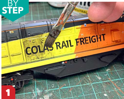
1 Work began with a coat of enamel weathering wash brushed onto a section of the body with a soft, flat brush, working the pigment into all the nooks and crannies.
