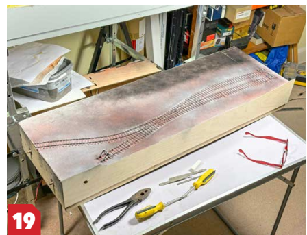
19 Once the power connections were correct and working well, it was time to paint the track using a mix of red, black and grey Halfords aerosol primers (work outdoors if possible). The primer also seals the paper surface of the foamboard.
