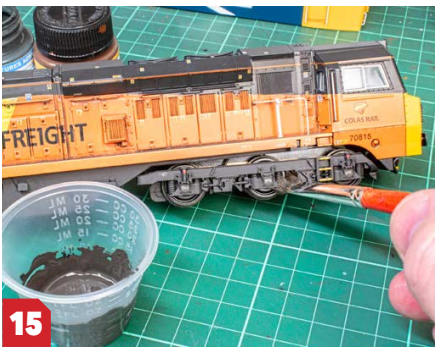
15 After re-fitting the cabs, weathering continued. A blend of LifeColor acrylics was created and stippled over the chassis and bogie frames. The exact colour is not critical at this stage.
