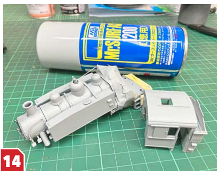
14 After cleaning up the body sections, I masked up the cab interior and rear bufferbeam before spraying a couple of light coats of Mr Surfacer 1200 grey primer. This was left overnight to harden completely.
