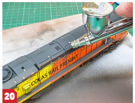
20 Switching to the Weathered Black shade, the roof and upper areas of the body were misted, concentrating around the exhaust outlets and introducing some streaks.
