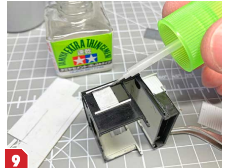
9 A similar set of sliding shutters and rails was cut and fixed to the cab's side apertures. Again, scraps of plastic, saved from previous projects, provided the materials - proving that it's worth holding on to offcuts for future use.
