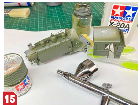
15 In a nod to the Bosnian Class G2, I fancied a light green livery, although a dark green shade was applied first. Tamiya XF-81 RAF Dark Green was thinned slightly and airbrushed over the tanks, boiler and cab.
