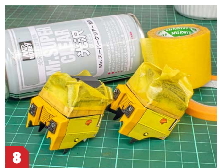
8 I masked up the glazing and sprayed the side panels and nose ends with two light coats of clear gloss - I used Mr Hobby's Mr Super Clear aerosol, which produces a tough finish.
