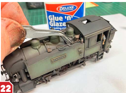
The weathering paints were left to dry fully before the model was carefully reassembled. Various fire irons, oil cans and tools, from the Modelu range, were fixed to the top of the tanks using Glue 'n' Glaze adhesive.
