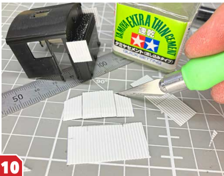
10 A sheet of corrugated styrene was marked out and cut to form a simple extension for the bunker. I trimmed the material imperfectly, to mimic panels that have been bolted together. Little touches like this add oodles of character.
