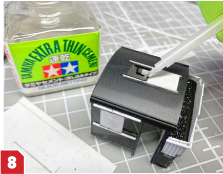
8 Using offcuts of thin styrene sheet and strip, I fashioned a sliding roof vent cover and rails, fixed in position with Tamiya's Extra Thin liquid poly cement, using the fine brush supplied. This cement creates a very strong bond.
