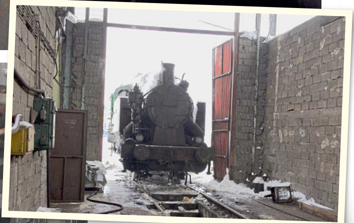
Above: The engine shed is of basic breeze block construction. Working industrial railways do not offer pristine surroundings - as demonstrated by the various pieces of equipment in this scene.
