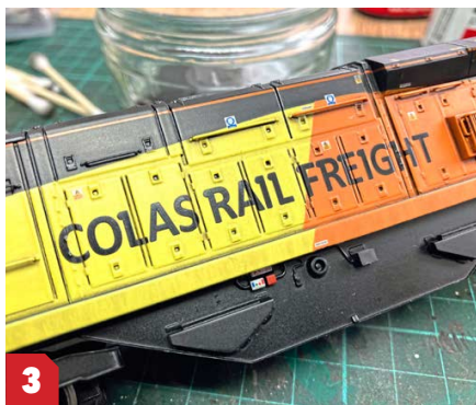
3 You can remove as much or as little of the wash as you deem fit. In this initial treatment, the sides have been cleaned up quite a bit, but the dark pigment is retained in the recesses.
