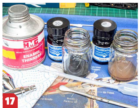
17 I thinned a pair of RailMatch enamel paints: Frame Dirt and Weathered Black. A small amount of each paint was decanted into jars and thinned to the consistency of skimmed milk.
