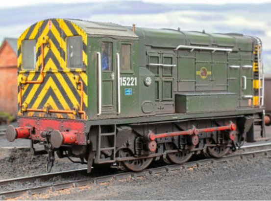
The weathering process has helped to highlight one of the Class 12s most unusual features: its larger Bulleid-Firth Brown cast metal wheels.
