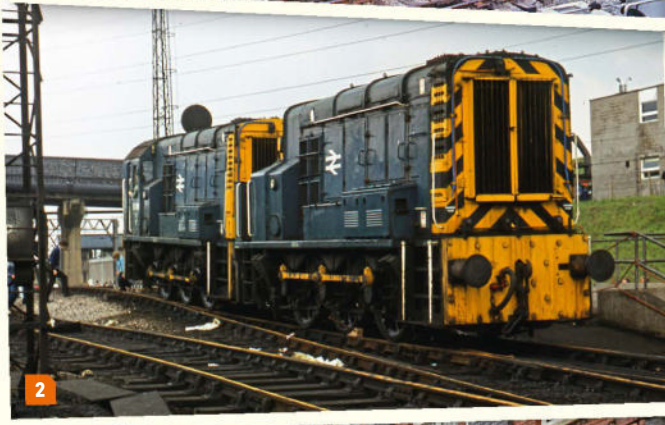
2: The Class 13s offered an ideal traction solution to cope with the pronounced hump at Tinsley Yard, as demonstrated by 13001, posing for enthusiasts in June 1980. COLOUR RAIL
