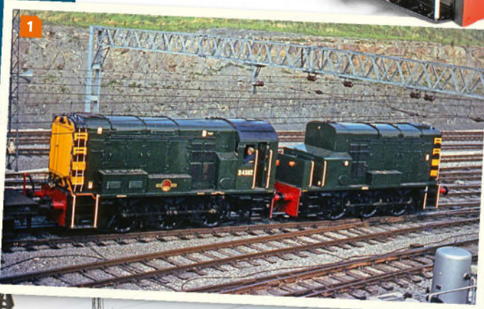
1: Initially, the Class 13 ensemble was coupled cab-to-cab, as modelled by newly converted D4502 at Tinsley Yard in 1965. COLOUR RAIL
