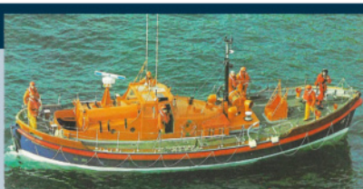
Above: The RNLB Duke of Cornwall , which I chose as the prototype of my model. It is seen here late in its career with the 1980s orange upper works, radar, and the distinctive cylinder for the self-righting air-bag on the rear cabin roof. ROYAL NATIONAL LIFEBOAT INSTITUTION
