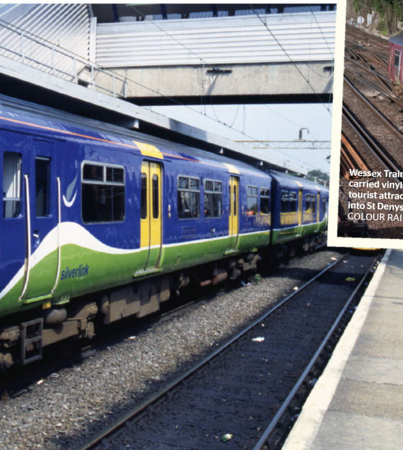
The early Class 150/2s originally lacked all-yellow ends and the gangway windows were later plated-over. COLOUR RAIL
