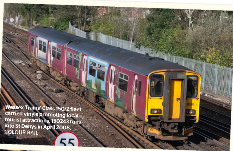
The early Class 150/2s originally lacked all-yellow ends and the gangway windows were later plated-over. COLOUR RAIL
