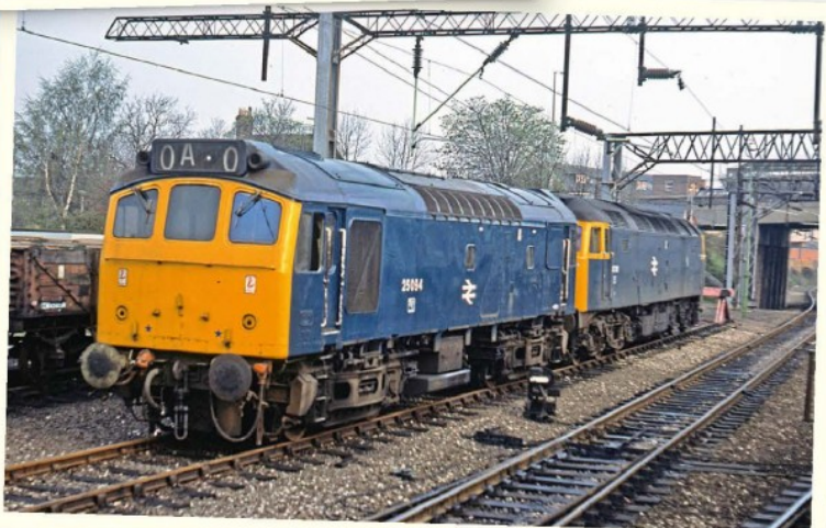
Below: Stabled near Stafford station with a Class 47 for company, Class 25/2 25094 retains its alphanumeric headcodes in this 1978 view. The boiler vents have been plated over and the steam heat hoses removed. COLOUR RAIL
