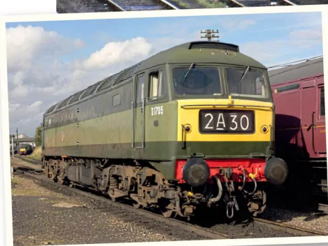
Returned to its original two-tone green livery, albeit without a retro-fitted Sulzer V12 power unit, D1705 is the sole surviving former Class 48, residing at the Great Central Railway. ALAMY
