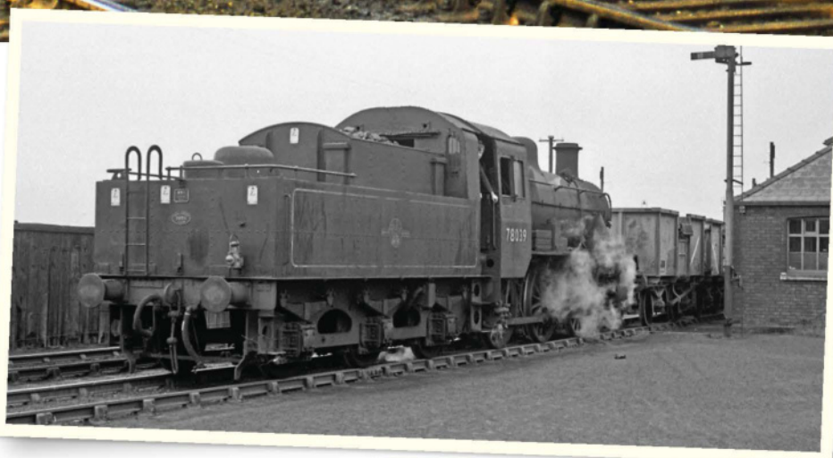
Right: The '2MTs' were designed to run tender-first when necessary, with good visibility afforded over the sides of the water tank. No. 78039 is working at Widnes in 1962. COLOUR RAIL
