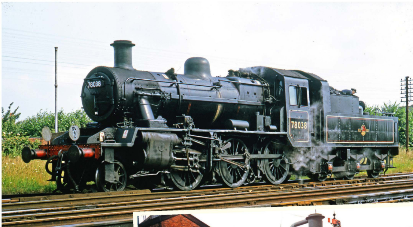
Above: In July 1964, No. 78038 is taking water at Shepperton. Note the flush coupling rods of the later-built '2MTs', compared to the fluted rods of No. 78000 below. COLOUR RAIL
