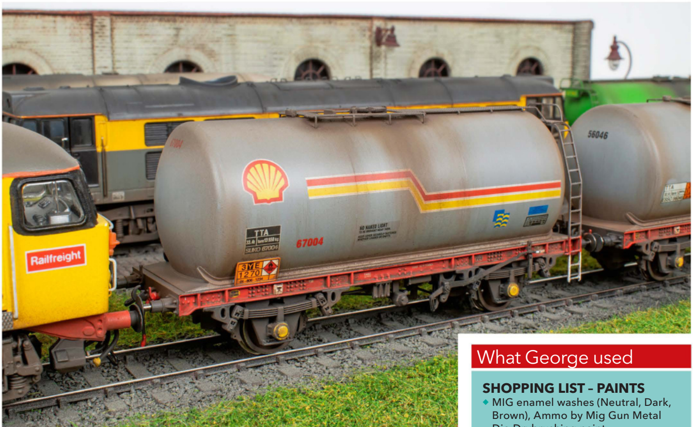
A layered weathering approach produces more lifelike results than a single application of paints or washes.
