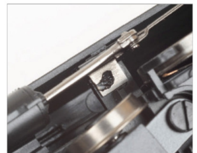
Hornby's 'West Country' and 'Battle of Britain' tooling dates back to 2001, retaining the same method of mounting the metal slidebars onto the plastic bracket.
