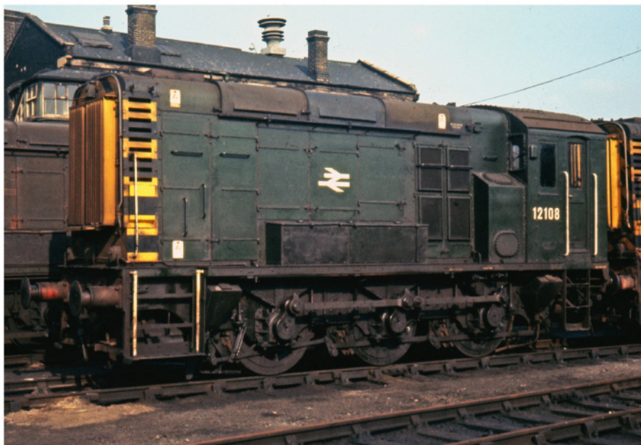
A rarity, in terms of livery, is seen here with 12108 in BR green livery with 'double arrow' logos, seen at Stratford in March 1968. Another interesting feature is the plain cab handrails, which lack the steam-era mounting knobs employed on many other Class 11s. COLOUR RAIL
