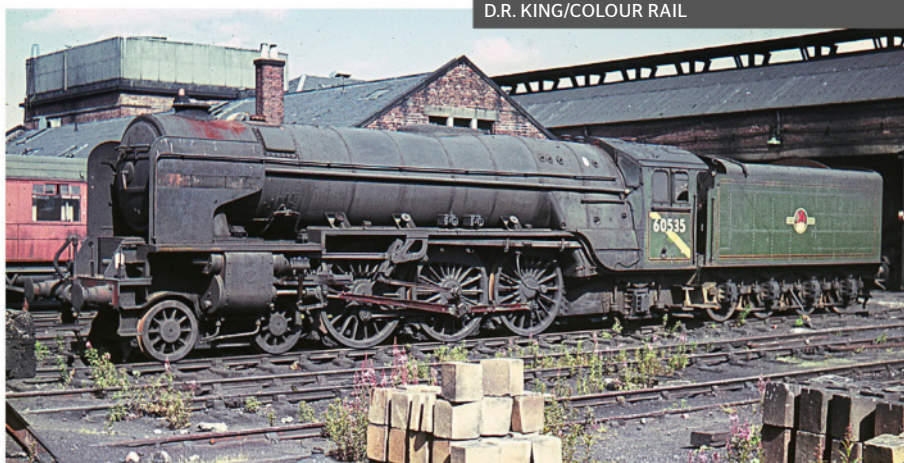
Below: A small number of Eastern Region 'Pacifics' carried the yellow diagonal stripes on the cab sides, denoting that they could not work south of Crewe on the newly electrified West Coast route - a somewhat unlikely occurrence by 1964, when the stripe was introduced. At least one Polmadie-allocated 'A2', No. 60535 plus 'A3' No. 60052 and 'A4' No. 60031, were so adorned. D.R. KING/COLOUR RAIL
