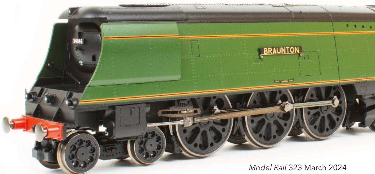
Hornby's 'West Country' and 'Battle of Britain' tooling dates back to 2001, retaining the same method of mounting the metal slidebars onto the plastic bracket.
