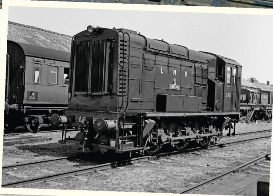
Right: Built by the LMS for the War Department, WD878 Basra stands at Longmoor shed on April 30 1966. War Department versions of the 350hp 0-6-ODE carried large electric headlamps at each end. RAIL ARCHIVE STEPHENSON
