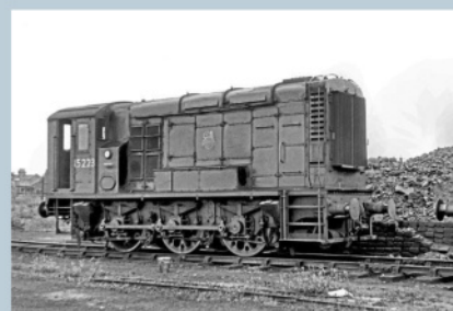
Below: 15221/212 stand at Hither Green in June 1970. Electric lamps were a later addition, with 15223 (above) showing the original layout of lamp brackets. 'Boxpok' wheels (above left) were a distinctive feature of the Class 12s.
