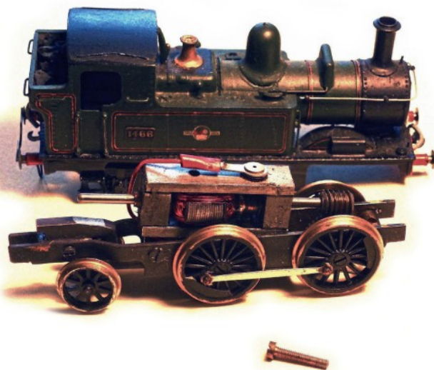
The chassis of a K's '14XX' 0-4-2T fitted with the earlier three-pole motor and no flywheel. CHRIS LEIGH
