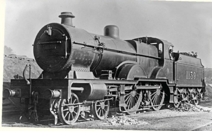
Above: One of the low-pressure outside cylinders is prominent in this view of nearly new LMS No. 1139, which was built by the North British Locomotive Company in 1925. COLOUR RAIL
