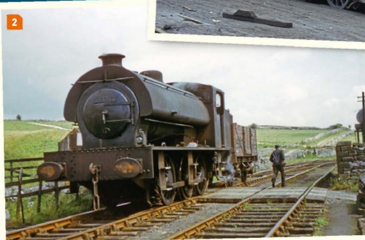
1: A grimy 'J94' No. 68053 rests at Darlington shed, August 1964. Note the extra set of footsteps and handrail on the saddle tank - features included on the BR versions of the EFE Rail 'J94'. COLOUR RAIL
