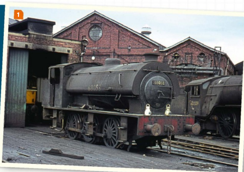
1: A grimy 'J94' No. 68053 rests at Darlington shed, August 1964. Note the extra set of footsteps and handrail on the saddle tank - features included on the BR versions of the EFE Rail 'J94'. COLOUR RAIL
