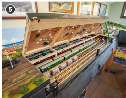
All of the electronics underneath the liftable baseboards are mounted within the 2x1 frame so that the components can be worked on without having to clamber underneath.
