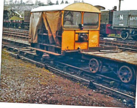
This Wickham trolley sports the 1980s-era livery of all-over yellow and pale roof. The side curtains could be folded down to provide a modicum of protection for those inside. CHRIS LEIGH
