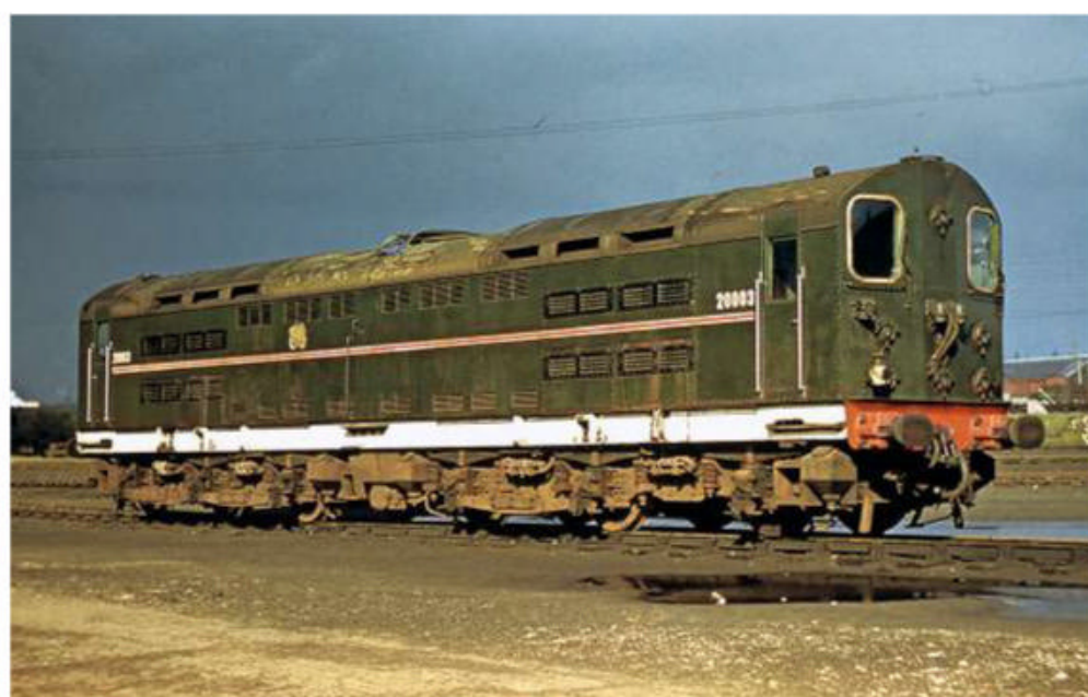
Right: The Southern followed a different scheme for its electric locomotives, with this handsome green scheme eventually emerging. A red and white horizontal band was added at waist height along with a pale grey stripe on the solebars. BR emblems were also added, although SR 750V DC Co-Co No. 20003 seems to be missing the crests in this view. B. SWAIN/COLOUR RAIL
