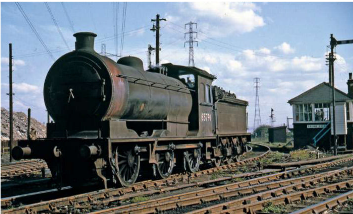
Above: Another view of No. 65894 prior to its preservation career, sharing space with Sulzer Type 2 and English Electric Type 4 diesels at York shed. The short dome, overhead line warning legends and twin-railed bunker are noteworthy. Many 'J27' tenders featured three coal rails. York's 'J27' fleet appear to have been kept relatively clean and lacked the rusty/burnt smokeboxes of those employed further north. COLOUR RAIL
