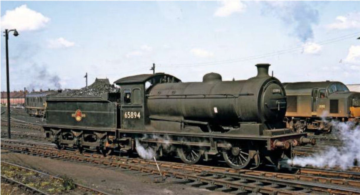
Above: Another view of No. 65894 prior to its preservation career, sharing space with Sulzer Type 2 and English Electric Type 4 diesels at York shed. The short dome, overhead line warning legends and twin-railed bunker are noteworthy. Many 'J27' tenders featured three coal rails. York's 'J27' fleet appear to have been kept relatively clean and lacked the rusty/burnt smokeboxes of those employed further north. COLOUR RAIL
