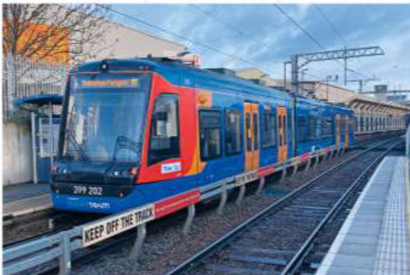
Above and below left: Here’s what a joint tram-train station is all about: twin-height platforms, low-level for trams and normal height for trains.
