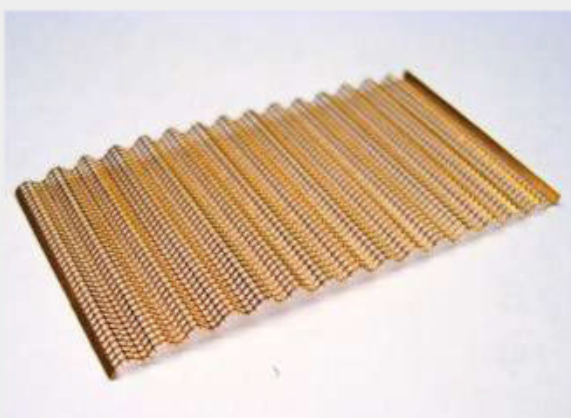
Having cut a piece of the grill to size (exact height, but slightly too long), it can be rolled through the Corrugator tool. Once shaped, the grille can then be cut to the correct length.
