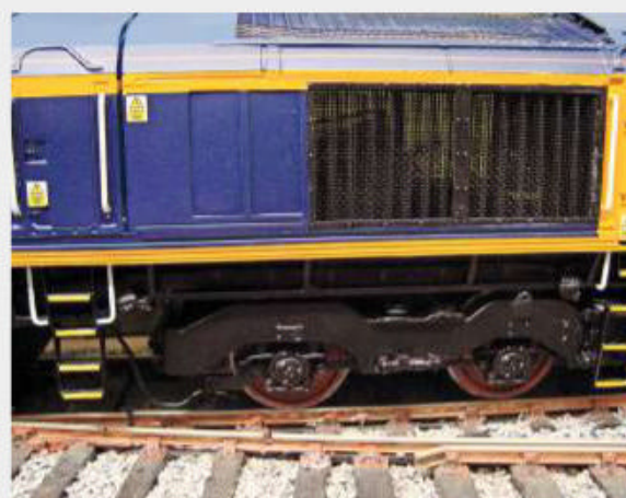
The new grille sections were painted black and then installed.
