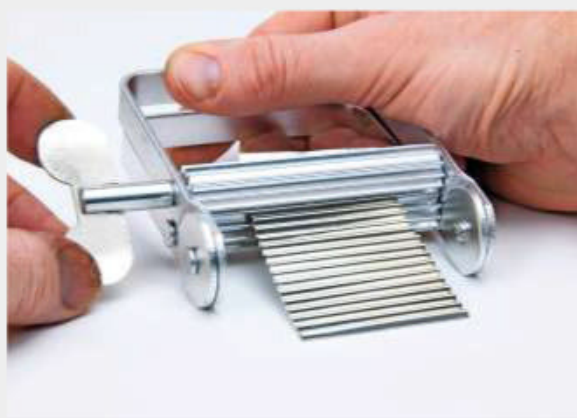
This is the magic Corrugator tool, from Green Stuff World, which can be used to form corrugated profiles in all sorts of materials, including thin metal sheet.
