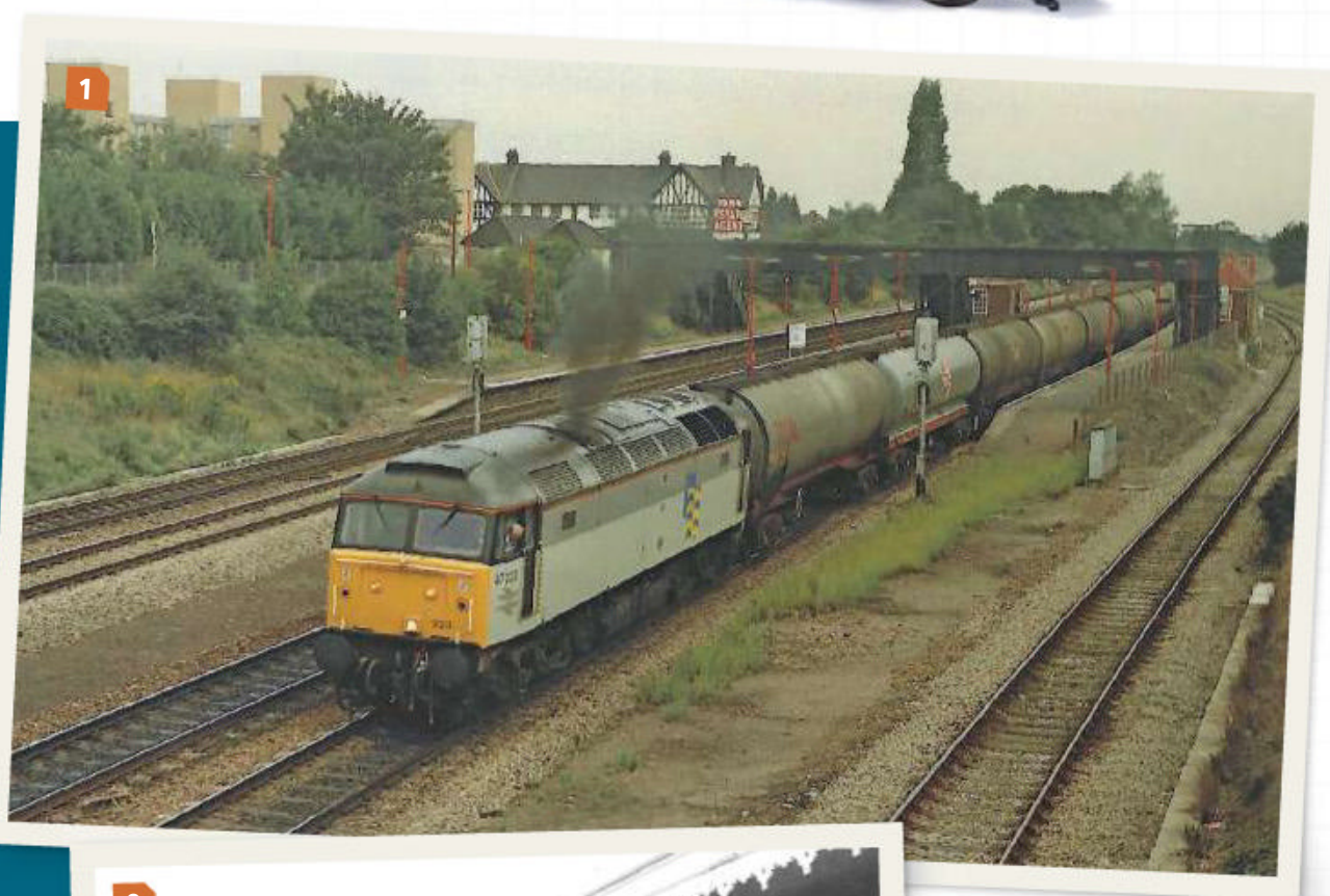
1: The Serck shutters have opened as 47223 recovers from a signal slack at Iwer with the Langley-Lindsey refinery aviation fuel empties c.1991. It has standard marker lights at this end. CHRIS LEIGH
