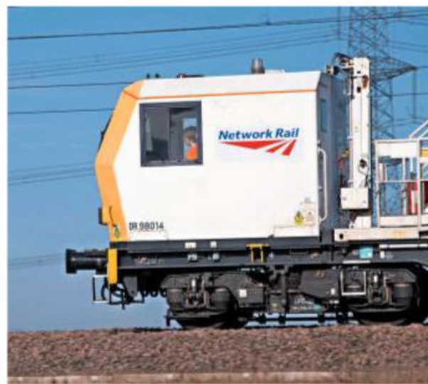
Built for the West Coast Route Modernisation scheme, Windhof electrification vehicle DR98014 is seen on the WCML near Lichfield Trent Valley in 2016. ALAMY
