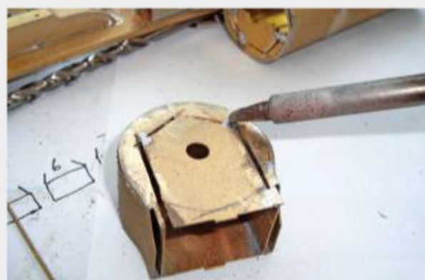
After each cut was made, a solder tack joint was added to hold the parts in place. This also helped to retain structural integrity and avoid any distortion of the smokebox assembly.
