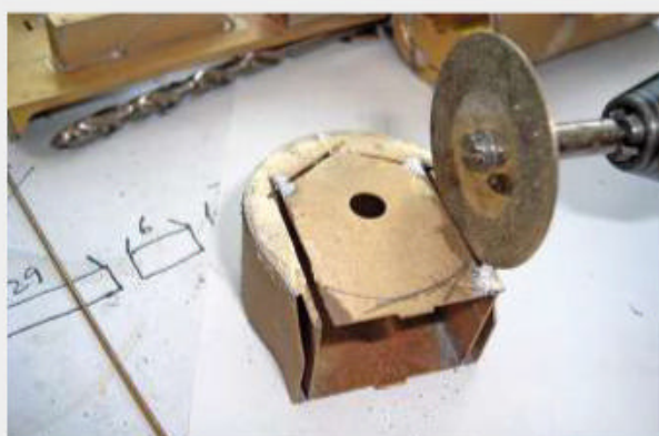
Using a slitting disc in a miniature power drill (don't forget to wear eye protection), a series of cuts were made into the inner smokebox former, just big enough to give clearance for the intended smoke unit.
