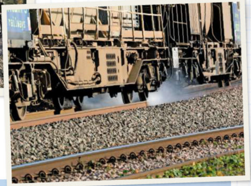
Right: During the leaf fall season, Network Rail's fleet of MPVs are employed to clear the rails of slippery debris using high-pressure water jets. ALAMY
