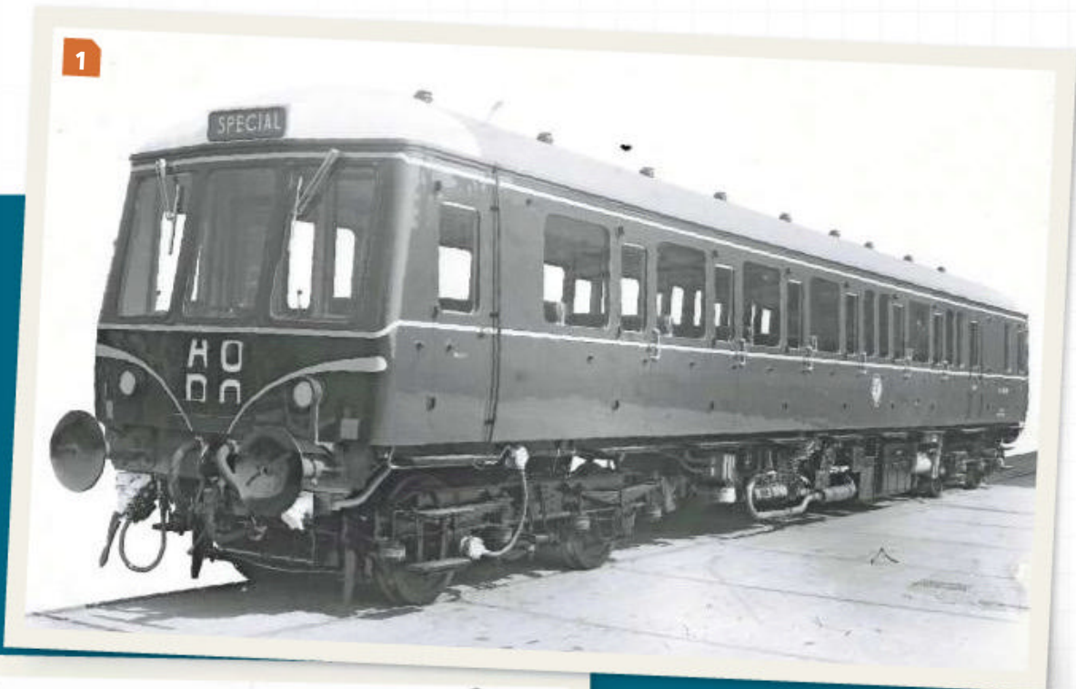
1: The official Swindon portrait of GRCW (Class 122) railcar No. W55000 shows the 'tidy' end, without the exhaust pipes. BR/CJL COLLECTION
