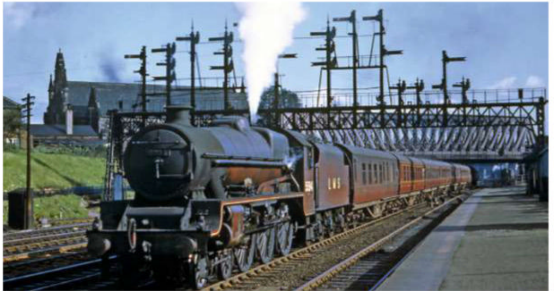
Below: An exception to lined black on the LMS is revealed by 'Jubilee' No. 5594 which received the traditional LMS red in post-war years. Seen here approaching York in 1949, with no sign of British Railways ownership, despite more than 12 months having elapsed since its establishment. E. SANDERSON/COLOUR RAIL
