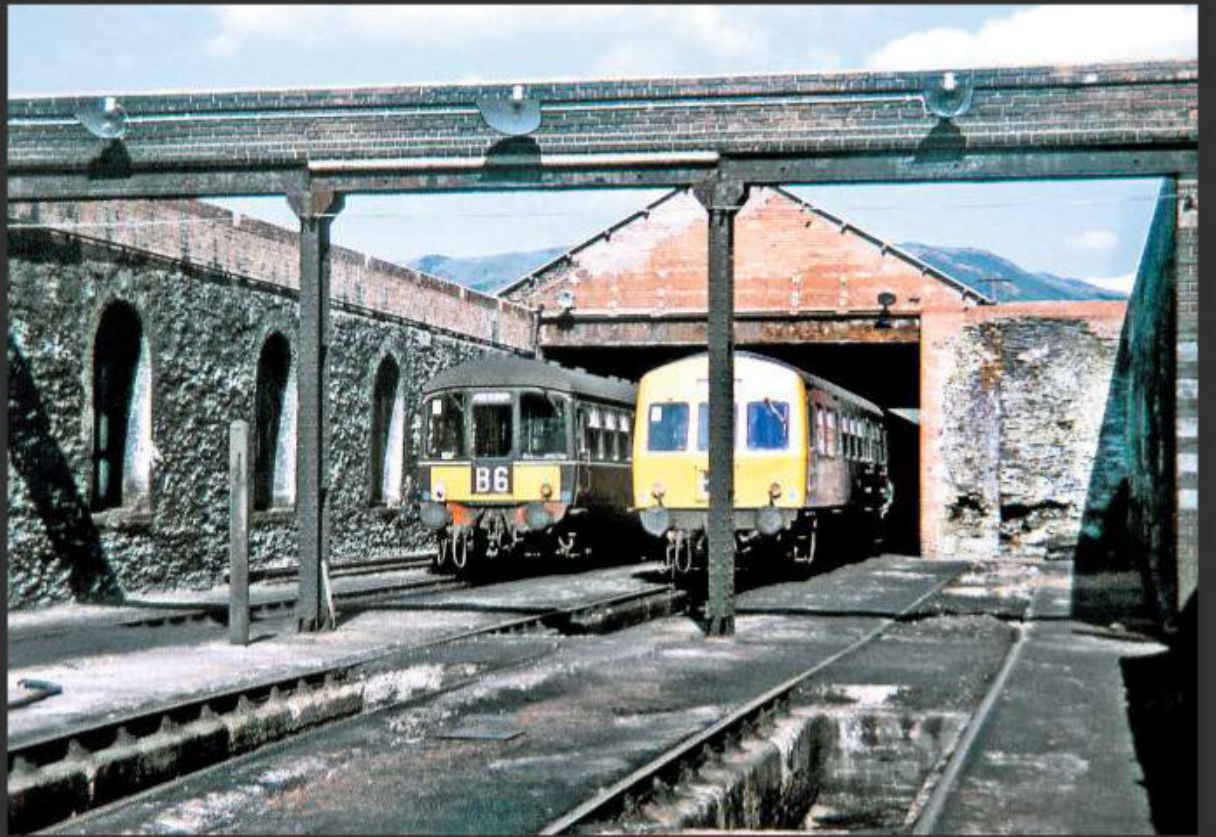
Park Royal Class 103 and Metro-Cammell Class 101 stand side-by-side in the former steam shed at Machynlleth, August 1968. A mix of local stone, brick and iron make for an interesting combination and the lack of a roof over part of the shed makes this a very modeller-friendly subject. RAIL PHOTOPRINTS
