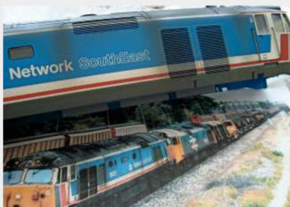
Always, where possible, start with a good clear photograph to use as a reference. The basic weathering was applied using RailMatch Frame Dirt (402), Executive Dark Grey (201) and Dark Blue/Grey (310).
