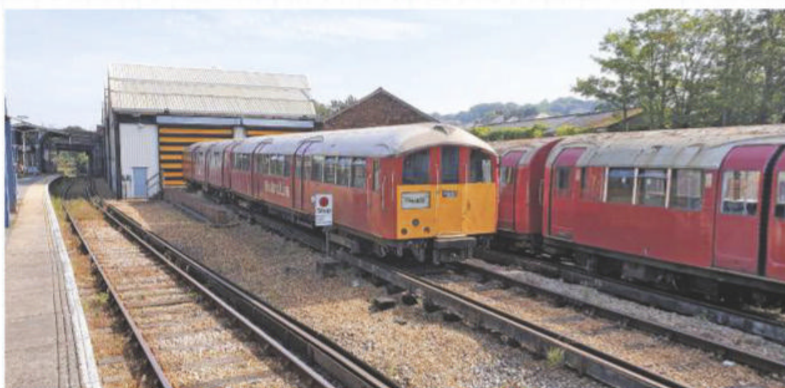
Above: On my most recent visit much of the 1938 stock was looking to be in pretty sorry condition, particularly at roof level. In terms of the main arrangement, the platform line is just a stub, ending some short way beyond the distant bridge. Note how the nearest track into the main workshop was raised (in 1988) to give better access to the traction motors of the former Underground stock.
