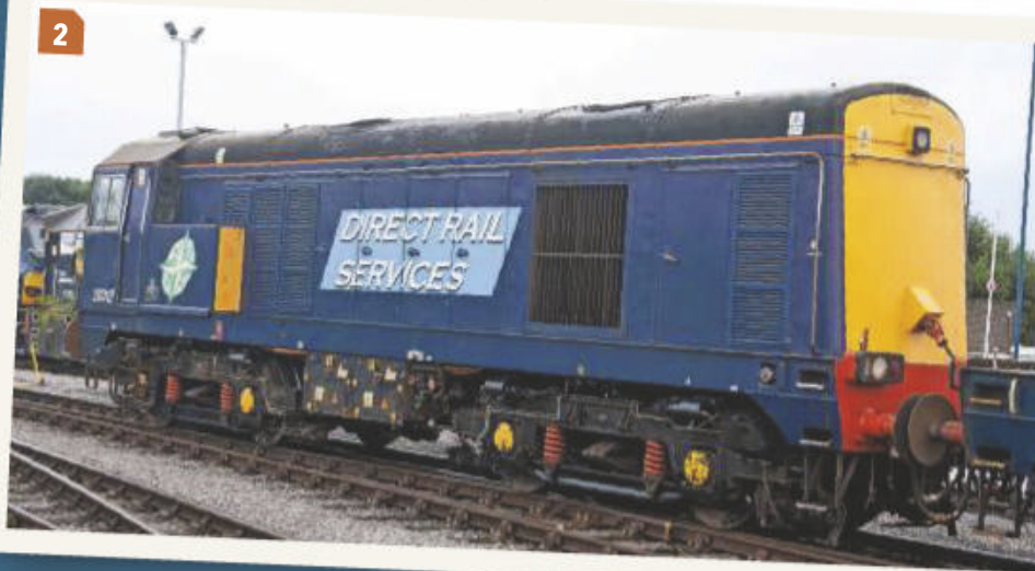
1: As one of the initial batch of Class 20/3 conversions, 20302 lacks the upper, central headlamps.
