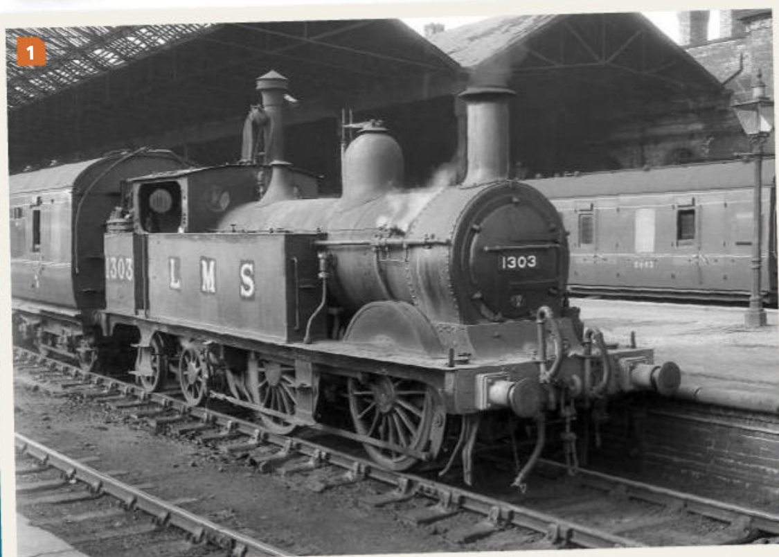
1: No. 1303 has had its LMS lettering and number wiped over but still carries a layer of grime everywhere else as it waits at Derby station in this 1940s photograph. The '17A' shedcode is for Derby shed. The LMS fitted the '1532s' with push-pull gear for working motor trains. RAIL ONLINE
