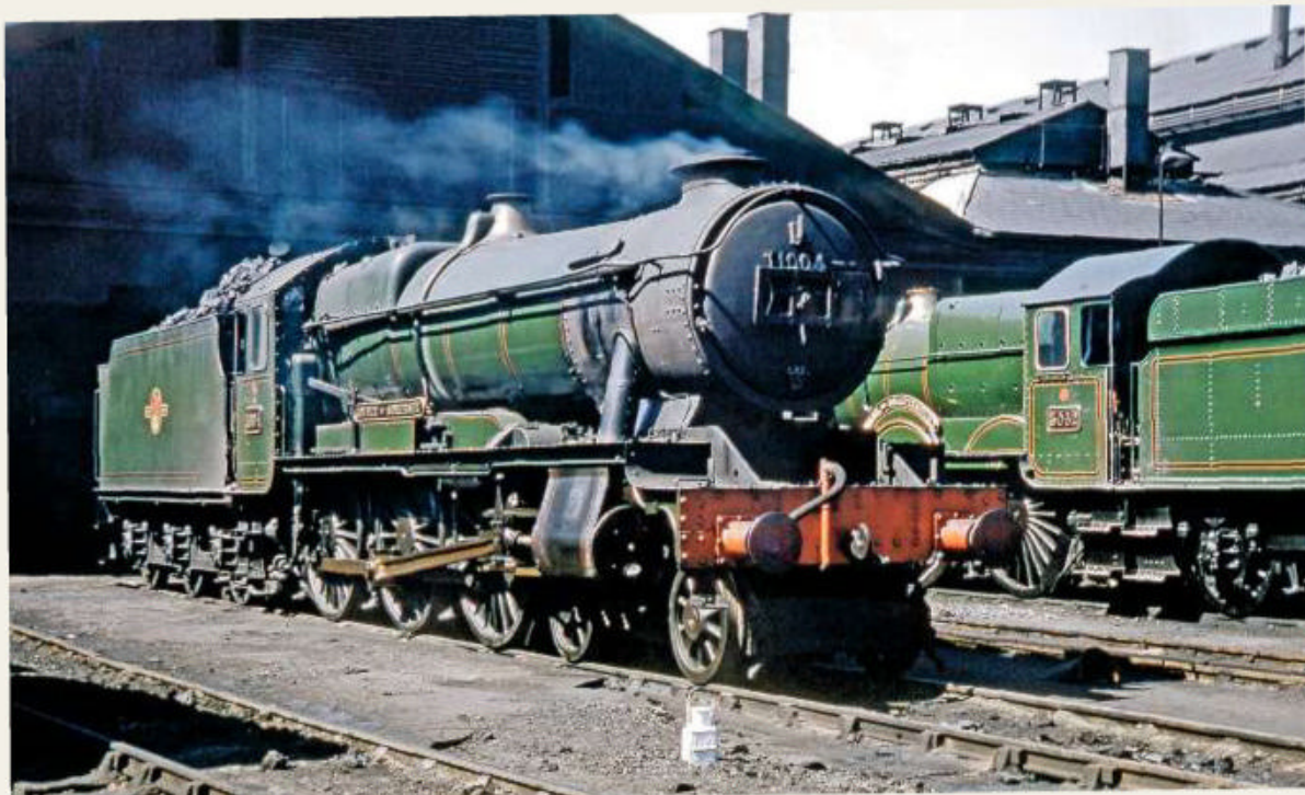
No. 1004 County of Somerset glints in the sun outside Swindon shed on June 16 1957, alongside 'Castle' No. 5062 Earl of Shaftesbury . The straight nameplates on the driver's side were fixed to a mount to clear the reversing rod. DAVE COBBE COLLECTION/RAIL PHOTOPRINTS
