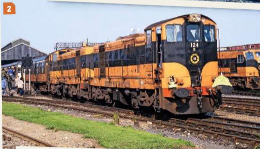
1: B121 carries CIÉ's grey/yellow livery as it shunts Mullingar in June 1961, shortly after delivery from General Motors. The class were delivered with 950hp 8-567 engines and louvres on the solebar but no solebar handrails. COLOUR RAIL
