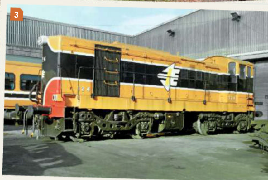
2: '121s' 124 and 122 stand at Limerick with a railtour on September 13 1986. Work had started to equip the '121s' with 1,100hp engines. The solebar handrails are visible, as are the multiple working sockets just above the buffers. BERT WYNN/RAIL PHOTOPRINTS
