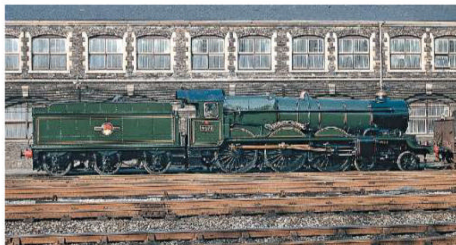
Above: Fresh out of Swindon Works, 'Castle' No. 4077 Chepstow Castle's wheels have been painted black but the rods were left burnished - and soon gained a layer of surface rust. The handrails are 'body colour' - 'Kings' had them burnished - the brightwork is polished and the post-1956 BR coat of arms is centred on the tender panel. BILL POTTER
