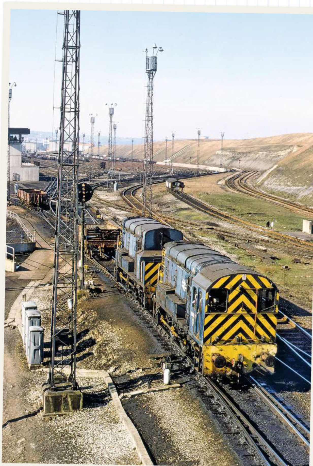
Above: The Dowty hydraulic retarder gear – just visible in front of the hybar wagon – gave the Class 13s severe wheel flats. Therefore the Class 13s had their tyre profile modified. This work was undertaken at Doncaster Works, with the Class 13s running to and from the works under their own power. LES NIXON
