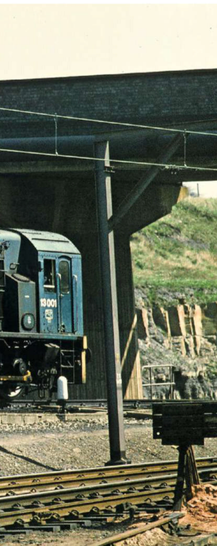
Above: The Dowty hydraulic retarder gear – just visible in front of the hybar wagon – gave the Class 13s severe wheel flats. Therefore the Class 13s had their tyre profile modified. This work was undertaken at Doncaster Works, with the Class 13s running to and from the works under their own power. LES NIXON
