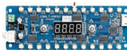
Fig 8: Alpha Mimic Panel Controller intercepts a command to a turnout and automatically illuminates the corresponding LED on the control panel.
