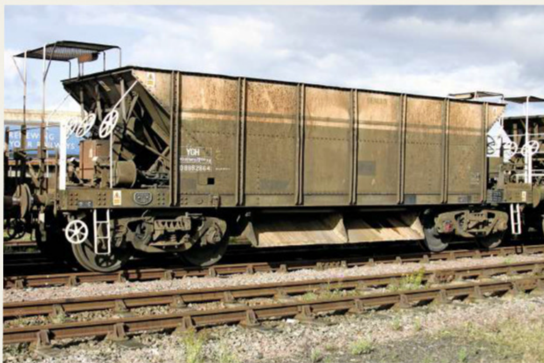
Below left: The grey panel, visible on the right hand platform, protects the electrical generating equipment fitted to 'Stingray' DB982892. ALL: GRAEME ELGAR
