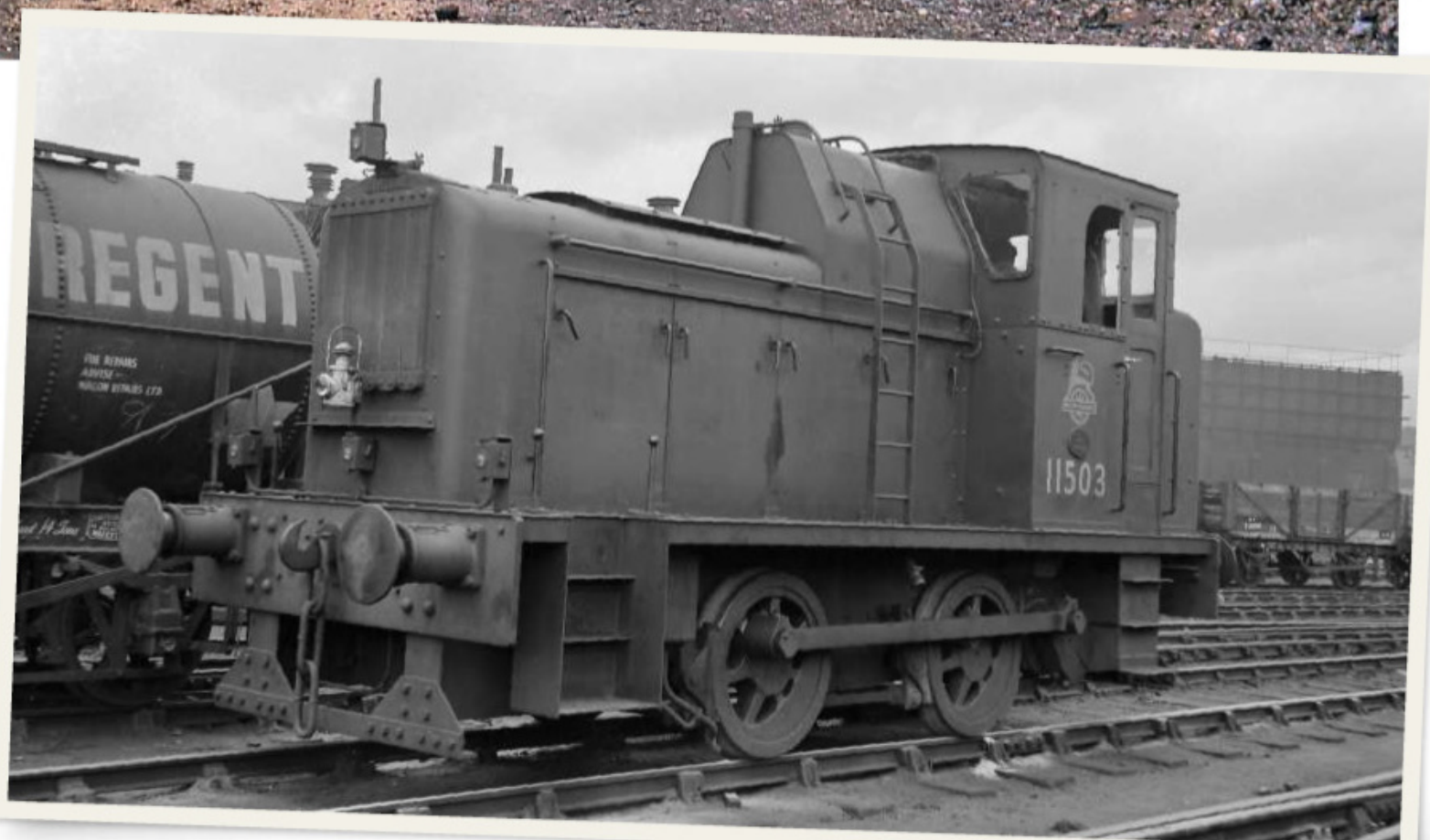
Above: D2955's work-stained paintwork has taken on a glossy sheen when it was photographed at Stratford in 1963. The slightly awkward shape was not helped by the fuel tank which was mounted atop of the bonnet, ahead of the cab. TREVOR OWEN/ COLOUR RAIL
