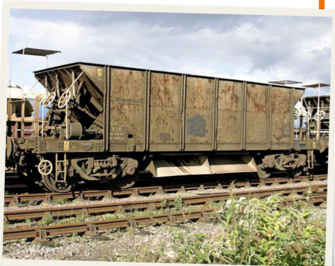
Above: 'Seacow' DB982550, coded YGB under the TOPS system, carries a very rusty patina in this 2006 view.
