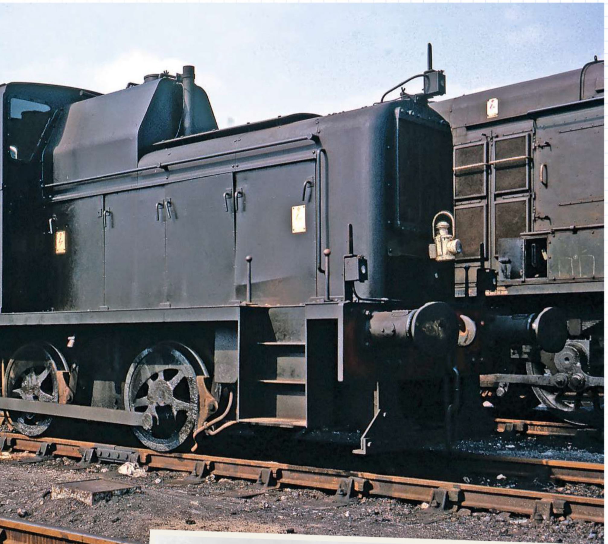
Above: D2955's work-stained paintwork has taken on a glossy sheen when it was photographed at Stratford in 1963. The slightly awkward shape was not helped by the fuel tank which was mounted atop of the bonnet, ahead of the cab. TREVOR OWEN/ COLOUR RAIL
