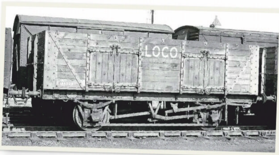
BR's mighty 'Transformer MC' No. B901800 stands in Bows Goods yard on December 29 1979. It was built by Head Wrightson to Diagram 2/470, Lot 2419, in 1953. PAUL BARTLETT
