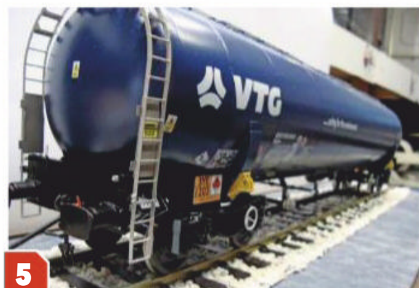
5 A fully finished ladder on a scratchbuilt 'Gauge 1' VTG TEA tank wagon that used the same technique as those for the PRMRP kit. Neither would have been possible to make without a block of wood.
