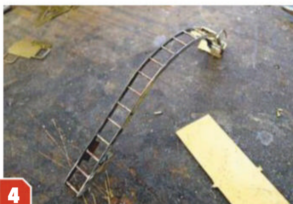
4 Then I used the disc to grind away the surplus brass and solder on the sides to leave the sides of the ladder smooth.
