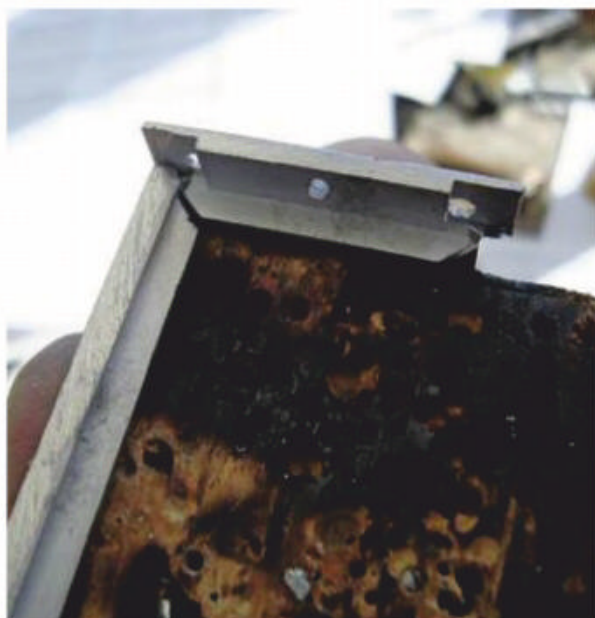
The block can be used to help when soldering large components together; these whitemetal castings come together to form the end and side of a 'OO' gauge tender.
