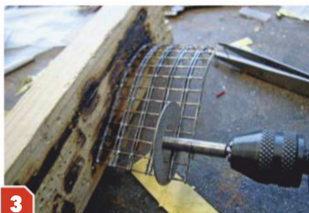
3 With all the rungs and side etches for 14 ladders soldered together, I turned the wood onto its side and, using a slitting disc in a mini-drill, I cut through the brass rods to separate the individual ladders.
