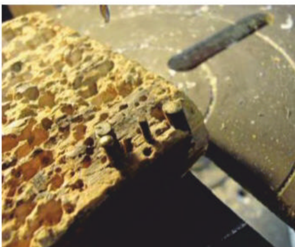
To stop the 4in by 1in piece moving around the drill base, I added a couple of screws that sit in the base slots.
