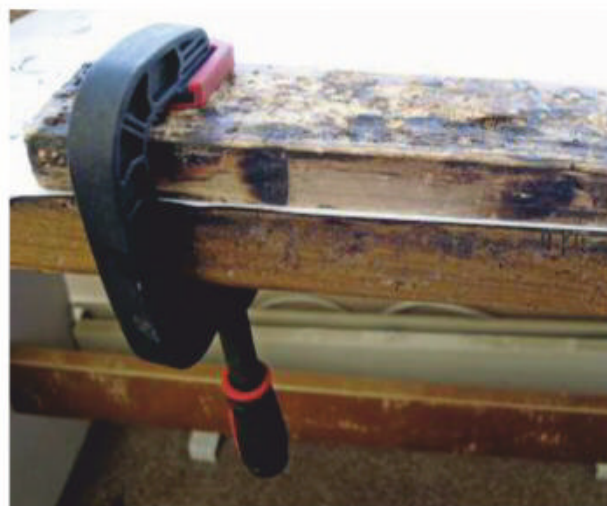
To help with stability, I clamp the 2in by 1in piece of wood to the work desk with a simple G-clamp. You can then hold down work pieces to the wood with drawing pins or more clamps.
