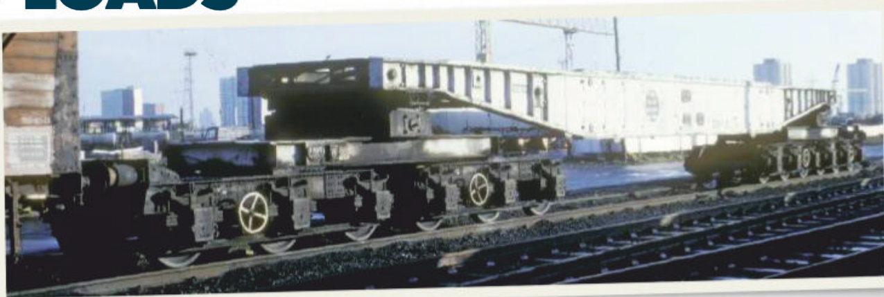
BR's mighty 'Transformer MC' No. B901800 stands in Bows Goods yard on December 29 1979. It was built by Head Wrightson to Diagram 2/470, Lot 2419, in 1953. PAUL BARTLETT
