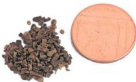
The gravel product may be more suitable for lineside piles of ballast and in a quarry, rather than being used as ballast, because the pieces are not a uniform size.
