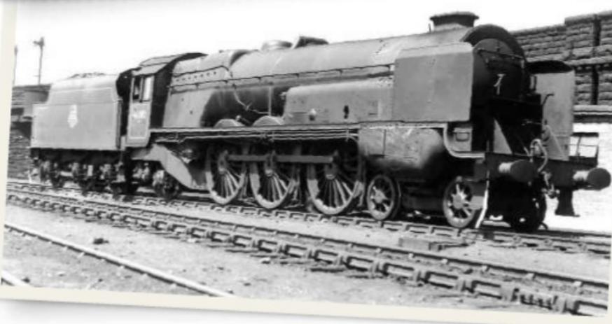
**Right: The ‘Turbomotive’ in BR lined black as No. 46202. It had carried LMS post-war black previously. The fairing over the reverse turbine has been extended. The turbine had failed in September 1935 and a new, stronger clutch shaft and inching gear were installed. MR COLLECTION**
