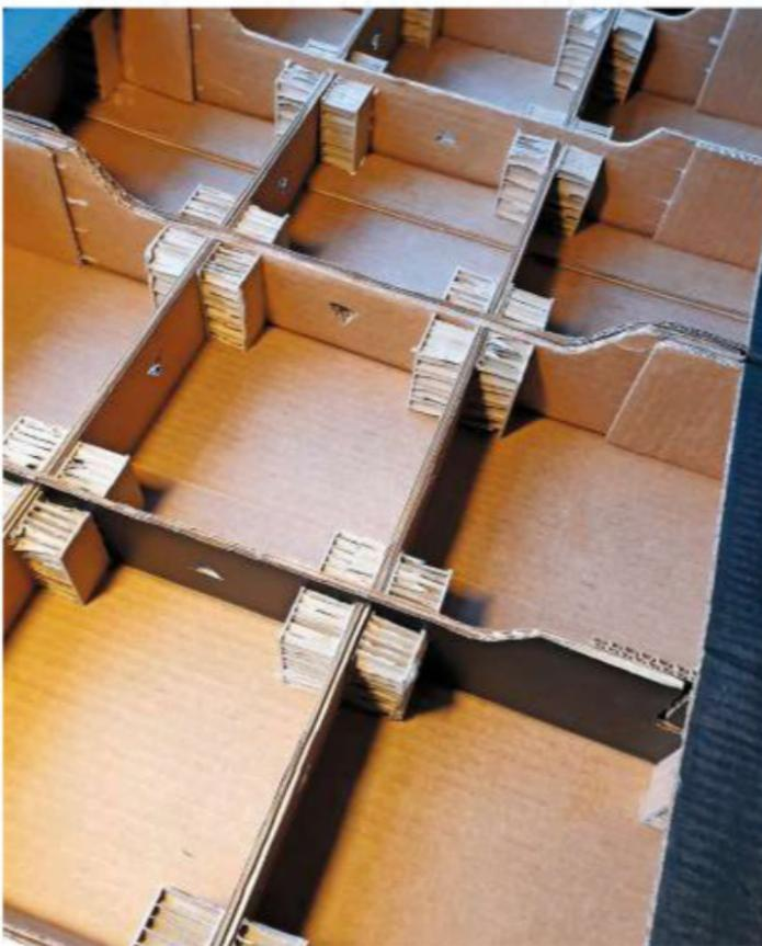
Above: Make and fit underside cross-member strengthening in both directions, with corner reinforcement at every joint. I used thick packaging card, though you could laminate thinner material as an alternative. Strive for constructional accuracy; a set square and sharp heavy-duty knife are essential and allow gluing to set overnight. Note the small triangular apertures in the cross-members for easy wiring.
