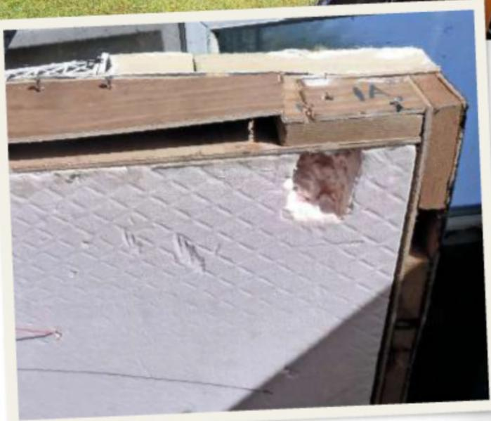
The partial collapse of the layout led to the slot-in leg tearing the plywood end out of one baseboard which had already been repaired once.
