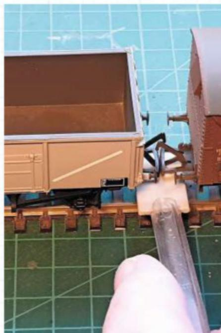
With limited funding there was no budget for point motors and a sophisticated uncoupling system. Here's my cheap and cheerful combination for both. I used a clear Bic pen barrel for point operation and, at the opposite end, a Tri-ang-type spatula for uncoupling - highly functional and zero (or minimal) cost. You might want to make a second version with the pen barrel and spatula at or near right angles for use in tight spaces close to vulnerable scenery.
