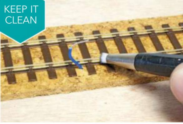
A reliable solder joint is only possible when both surfaces are clean. Tarnished or contaminated surfaces will prevent the solder from adhering correctly. Abrading metal surfaces with a glass fibre scratch brush can be effective prior to soldering, especially when fixing power feeds to the rails.
