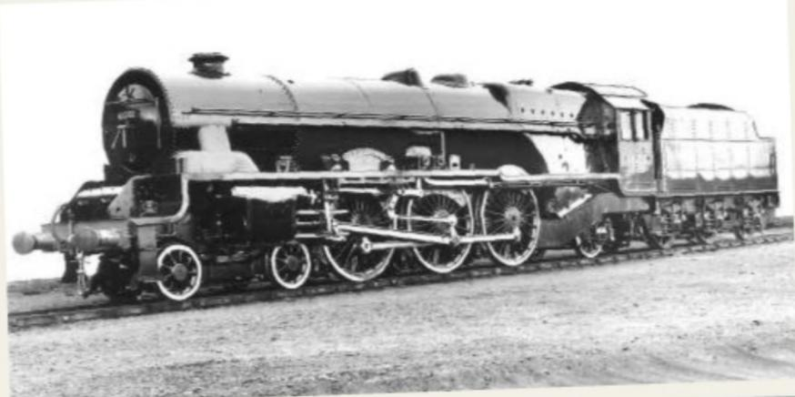
**Right: A works portrait of rebuilt ‘Turbomotive’ No. 46202 *Princess Anne* on August 13 1952. The front end is pure ‘Duchess’ while the rest, save for the stepped running plate, is ‘Princess’. Unlike the ‘Princesses’, the name plate is carried over the leading driving axle. MR COLLECTION**
