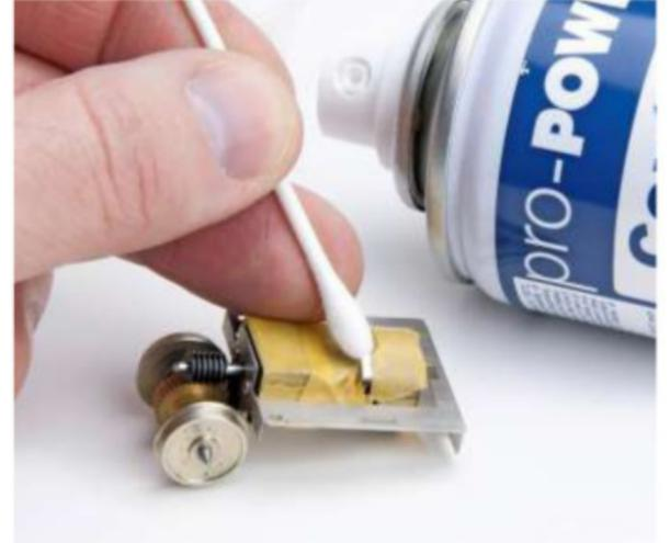
An alternative is to employ an electrical switch cleaning fluid, available from hardware stores. Decant a little fluid into a glass jar and use a cotton swab to clean the surfaces immediately prior to soldering.
