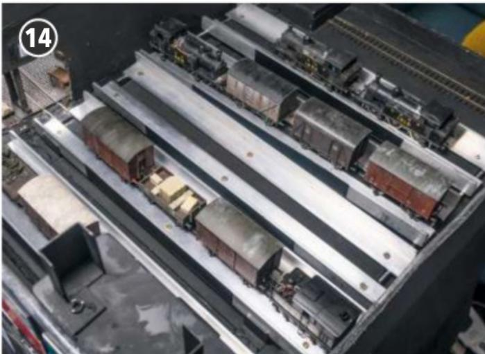
The 'live' end of the cassette fiddleyards sits on a strip of copper-clad sleeper as the main electrical connection and the locating lugs are also connected using bus bars. Some occasional adjustment is required, but they are generally quite efficient.
