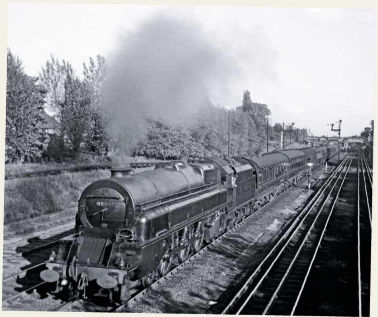
**No. 6202 speeds past Hatch End, Harrow with the Down 'Merseyside Express'. The locomotive always ran with the central lifting plate in the up position to maximise the air-flow into the lubricator cooler. The locomotive was nicknamed 'Gracie Fields' because the turbine whine increased with speed, giving the impression that No. 6202 was "singing as she goes". C.R.L. COLES/RAIL ARCHIVE STEPHENSON**
