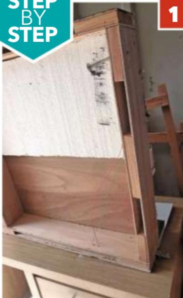
**1** The 'girder' end of an undamaged baseboard. It proved easy to remove the centre block of timber and replace it with a continuous strip of 2in by 1in timber, glued and screwed in place as a firm mounting for the hinged legs.
