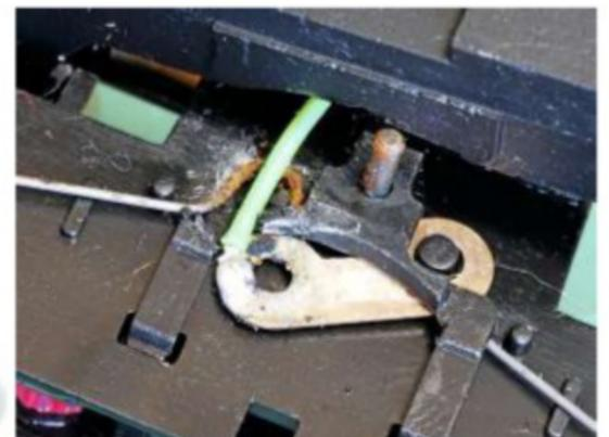
Poorly soldered joints and acidic flux residues not only lead to compromised electrical conductivity - they are also liable to mechanical failure.
