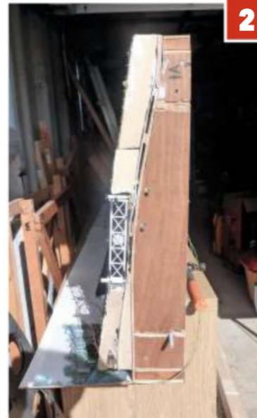
**2** The damaged baseboard end had served at three exhibitions with temporary repairs. I removed all the screws and broke away glued joints in order to use the broken pieces as a pattern for cutting a completely new end.
