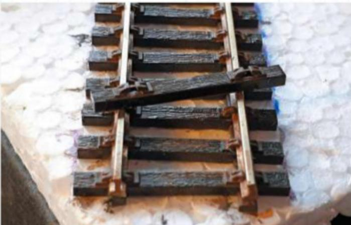
Above and below: I left a short section of track overhanging the baseboard edge on all lines. Those for operation were cut square and the disused line was cut at an angle to match the baseboard edge, using a cutting disc in a mini-drill.
