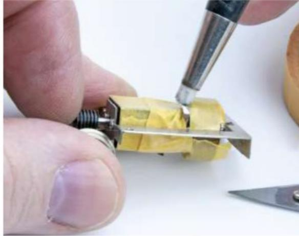
However, using abrasives near motors, gears and circuits can lead to contamination by metal particles and debris, so it's essential to protect these areas with masking tape. Once cleaned, don't touch the metal surfaces again before soldering.
