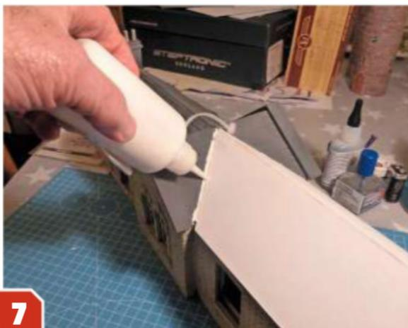
**7** I used Deluxe Materials Speedbond for gluing card parts such as the new roof sections, with Velo-Set adhesive to reinforce and fill some of the joints where a slightly more viscous adhesive was needed.
