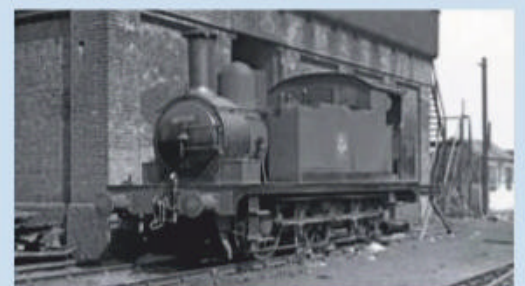
'J69/1' No. 68559 was built as an 'R24' with small tanks in 1895. It was rebuilt with a 180lb/sq in boiler and 1,200gal tanks in July 1904; pre-January 1904 rebuilds had 1,140gal tanks. K.L. COOK/RAIL ARCHIVE STEPHENSON
