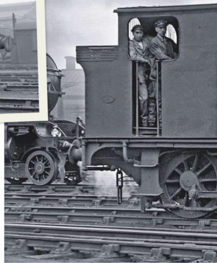
'J69/1' No. 7087 at Stratford shed in the 1930s. This was one of 14 'Buckjumpers' that BR inherited that were fitted with tripcocks for working freight services on London Underground's East London Line through to the Southern Railway via the Brunels' Thames Tunnel. RAIL ARCHIVE STEPHENSON
