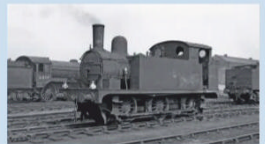
Shunting 'J69/2' No. 68513 at Stratford shed on August 10 1958. 'J69/2s' retained the small water tanks but with a 180lb/sq in boiler. 'J69s' had the whistles mounted on a stand-pipe in front of the cab. The line on the spectacle plate shows that No. 68513's wooden cab has been replaced with a steel one. K.L. COOK/RAIL ARCHIVE STEPHENSON
