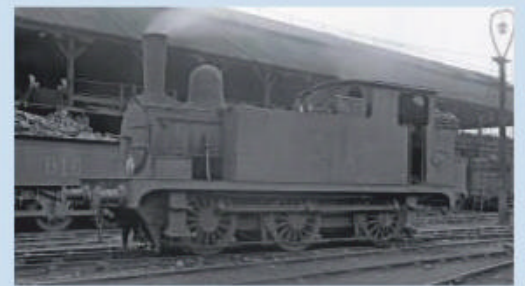
'J67/1' (GER 'R24') 0-6-0T No. 201 at Stratford shed, c1921. It has 1,000gal water tanks and 160lb/sq in boiler, identifiable with the safety valves in a bonnet over the firebox. It also sports the 15-spoke wheels (without balance weights) of the shunting version. WILFRED BECKERLEGGE/RAIL ARCHIVE STEPHENSON
