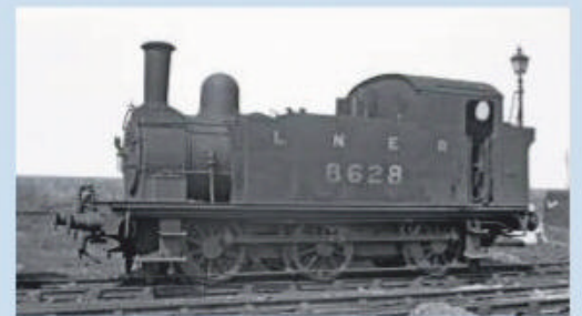
'J67/2' No. 8628 was built as a 'J69/1' in 1904. In 1938, it received a 160lb/sq in boiler and small firebox but retained its 1,200gal tanks and flush cabside. RAIL ARCHIVE STEPHENSON
