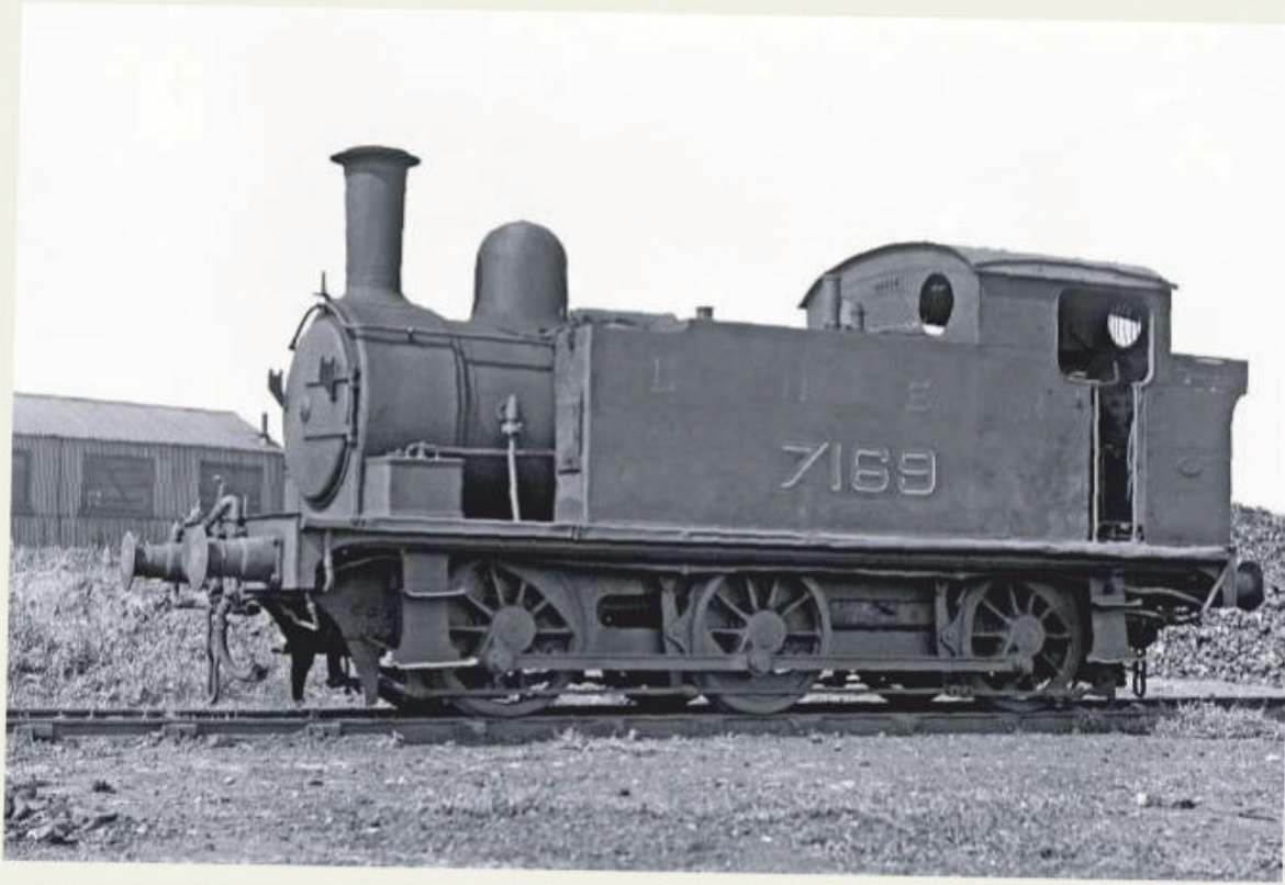
'J67' No. 7169 was loaned to the Government for use at Cairnryan, near Stranraer, between 1942 and 1945. Not only did it gain a modified chimney but it also received the LNER lettering and numbers in this odd, square typeface, possibly applied by the US military. A.W. CROUGHTON/RAIL ARCHIVE STEPHENSON
