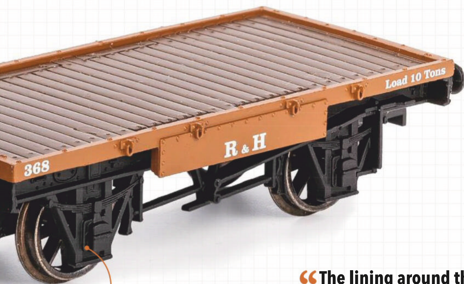
Additional electrical pick-ups (front axle of 'conflat')
