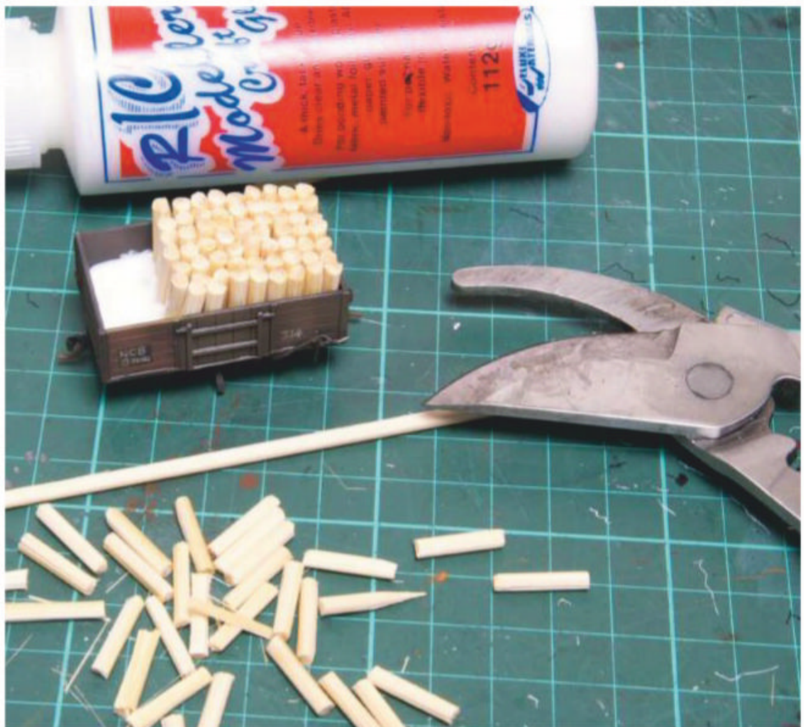
Above: Wooden barbecue skewers offer an extremely cheap and easy way to create authentic wagon loads, especially for pit props. Ideally, they should be treated with a dark wood dye before they're fixed into the wagon. GEORGE DENT
