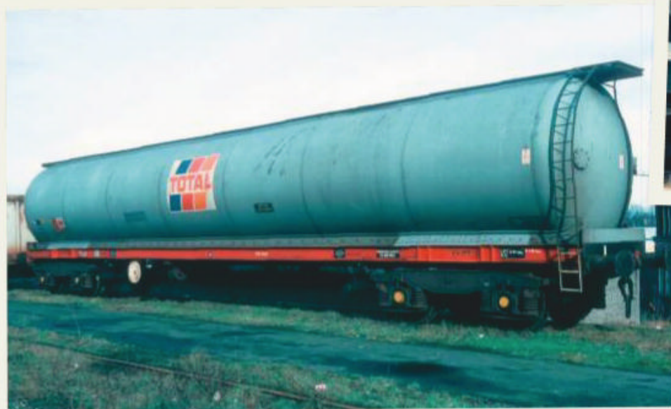
Above: A TEA Total Class A tank with Gloucester GPS bogies built to diagram TE009 standing at Standard Wagon works, at Heywood, on February 26 1989 and (above right) a 68t Bardon Hill Quarries PHA aggregate hopper built by WH Davis circa 1986 to design code JG010A, at Westbury, on January 13 1991. BOTH: PAUL BARTLETT
