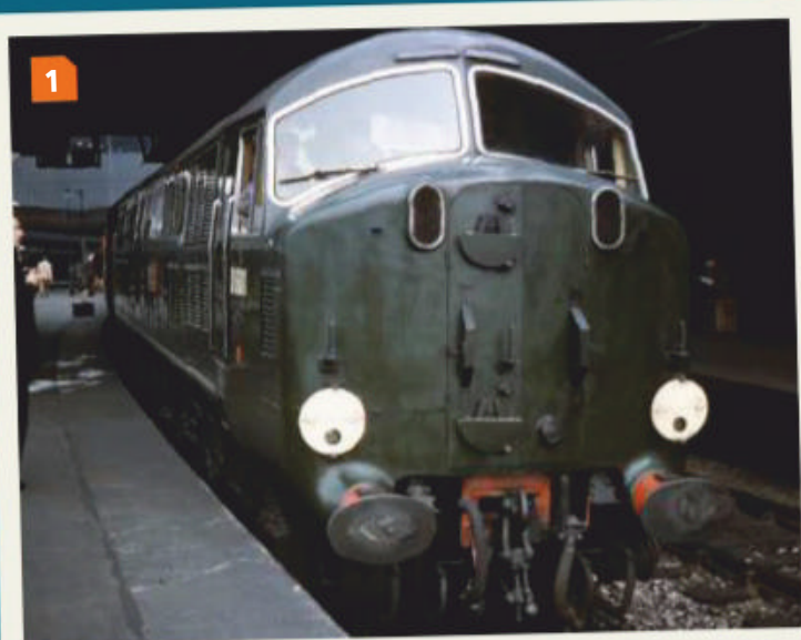
Above right: Pictured at Paddington early in its career, NBL Type 4 diesel-hydraulic No. D601 Ark Royal shows clearly the two additional mounting brackets which enabled it to carry a headboard or train reporting numbers. COLOUR RAIL
