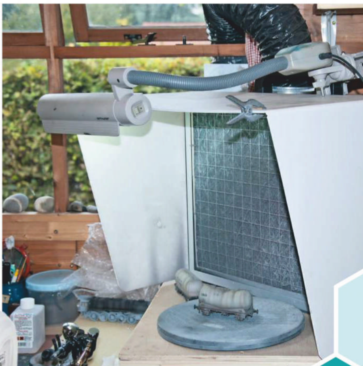
Above: A spray booth is recommended when airbrushing regularly. Be sure to replace the filters at the specified frequency.
