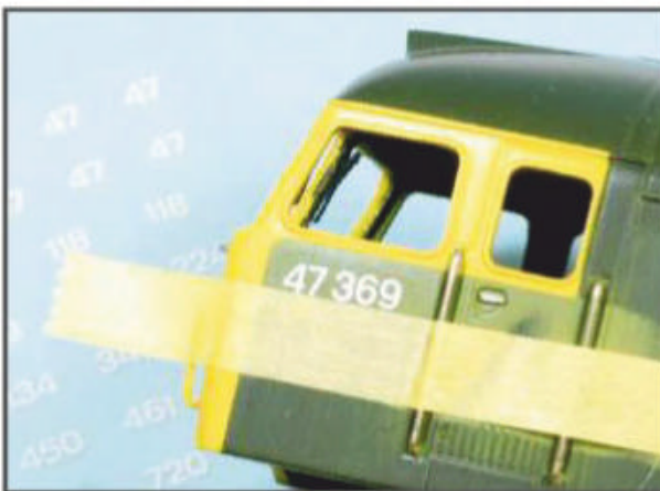
Rub-down decals are printed onto clear film, which helps you to accurately place the numbers.
