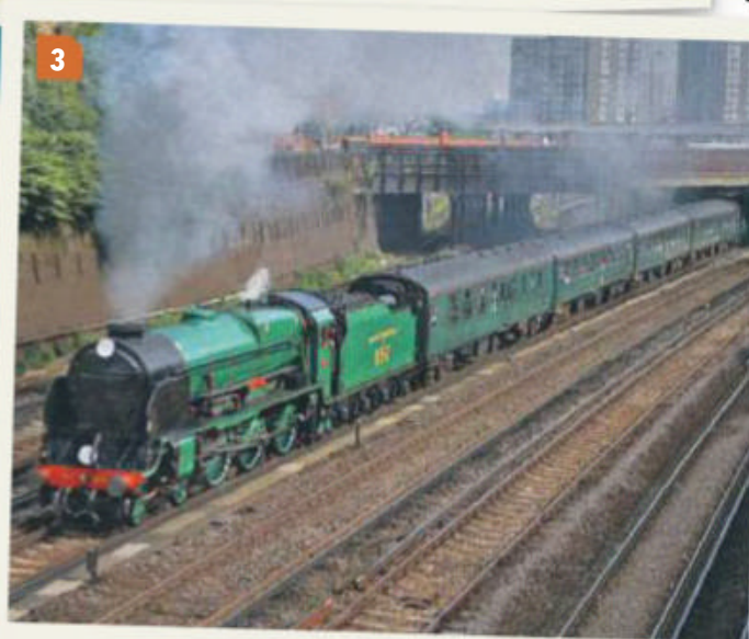
2: A stunning portrait of ex-works Sir Francis Drake , taken at Eastleigh. It has the Lemaître blastpipe, identified by the large diameter chimney and the post-1937 self-trimming tender. You can tell the latter by the raised raves. 'Drake' was unique amongst the 'LNs' - it received new cylinders but with 8in piston valves and, consequently, it kept its original length smokebox until withdrawal. COLOUR RAIL
