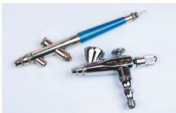
The trigger of a single action device controls the air, with paint flow governed by a screw at the tail end.
