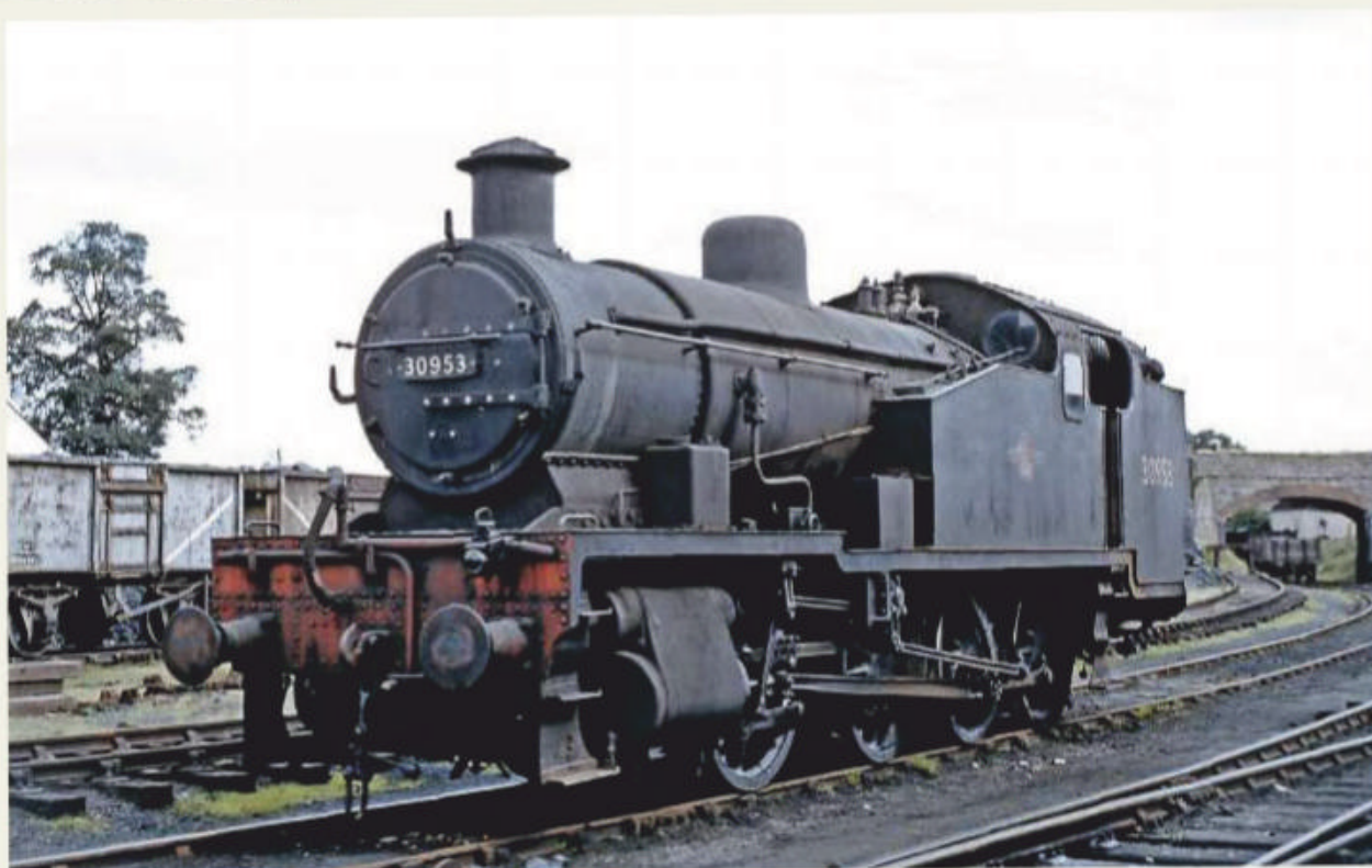
Below: No. 30953 at Templecombe shed on August 31 1958. As No. 953, it was the first 'Z' to receive the spare boiler that was built at Eastleigh in 1934. This boiler has extra washout plugs and fewer tubes. Existing boilers were later rebuilt with this revised tube layout. K.L. COOK/RAIL ARCHIVE STEPHENSON
