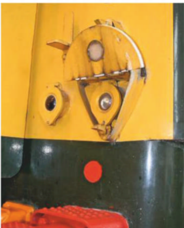
Headcode discs can be folded up (as here) or down, exposing the marker light behind and the unusual triangular framework around it.
