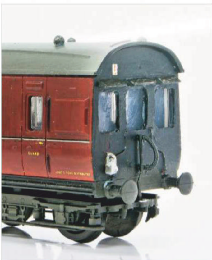
A trio of windows was cut into one end of the brake van to create the driving vehicle, along with a set of small, triangular sun visors over each aperture. The prominent curved gutter on the coach end was removed, and the raised guard's ducket should also have been flattened - but that was deemed a job too far. COLIN BOOCOCK
